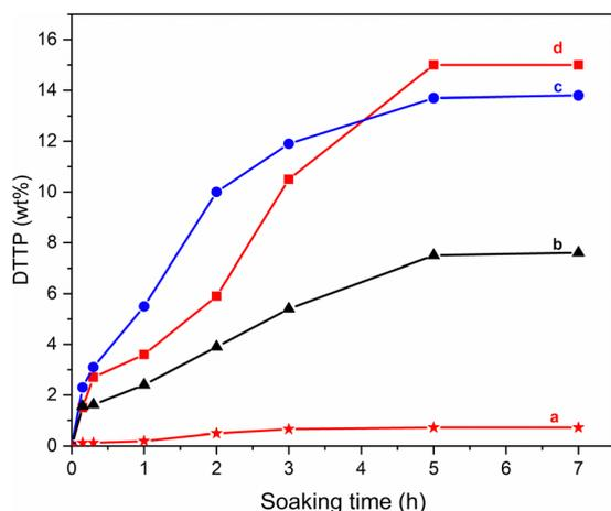
Fig. 6 DTPP release from B1/DTPP adduct: (a) obtained with silicon nitride (red curve, stars) in neutral solution, (b) tempered steel (blue curve, circles), (c) zirconia (black curve, triangles) and (d) Silicon nitride (red curve, squares), in acidic solution (pH = 1.3).
