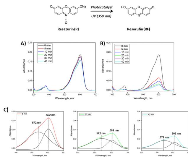
Fig. 10 Photocatalytic activity of COTTON-B1 (A) and COTTON-B1/DTPP (B) in resazurin aqueous solution under UV irradiation. (C) Deconvoluted spectra after 5, 20 and 40 min of reaction.
