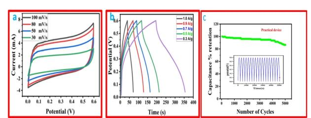
Fig. 8 (a) The CV curves of the practical device at various scan rates. (b) The GCD profile of the practical device (potential vs. time) at different current densities. (c) The percentage capacitance retention of a rMGO-GG/PVA-b based practical device as a function of number of cycles.
