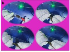
Fig. 3 (a) Effect of percentage content of rMGO on the electrical conductivity of the as-synthesized hydrogel composites of rMGO-GG/PVA-b. (b) The electrical conductivity stability of rMGO-GG/PVA-b IPN based composites undergoing the 180° twisting test.
