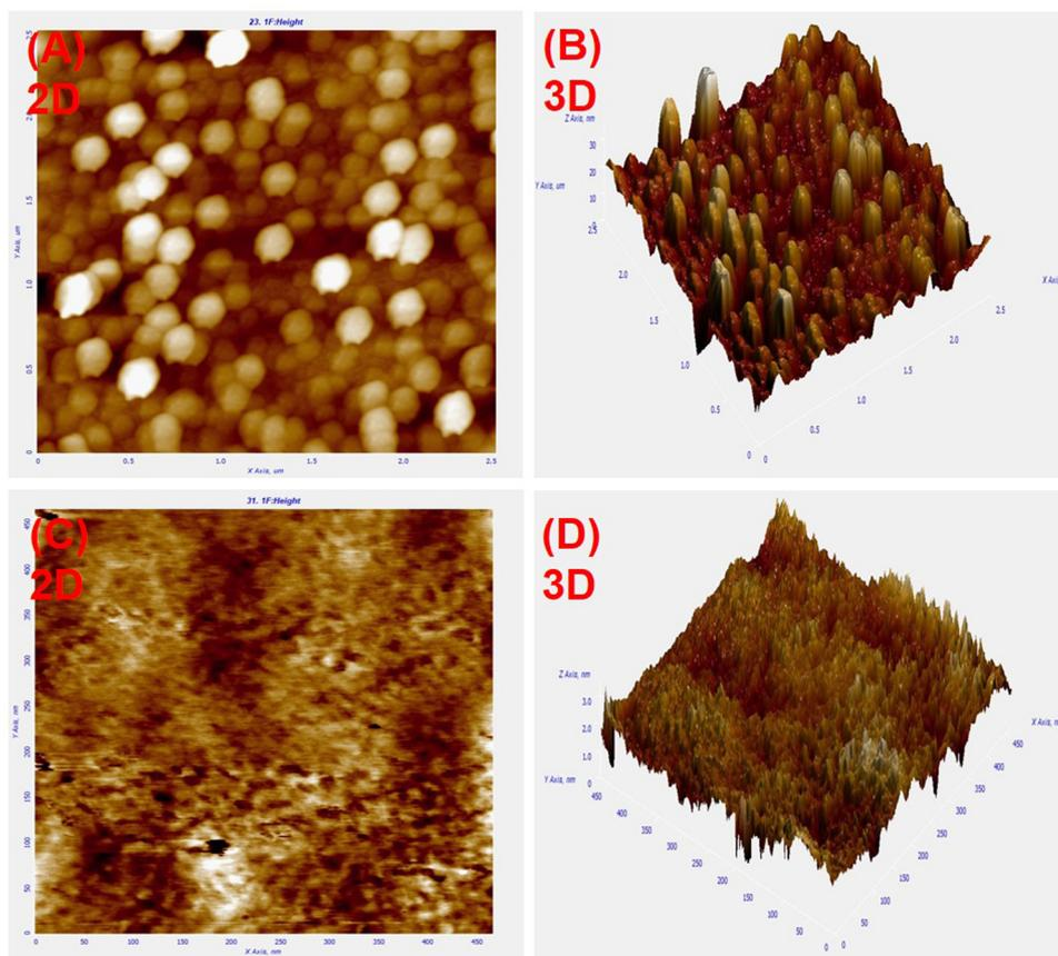
Fig. 4 (A) and (B) 2D and 3D images of AFM for the rare phase nanostructure  $\text{LaMn}_2\text{O}_5/\text{ITO}$  electrode. (C) and (D) 2D and 3D images of Tyr/ $\text{LaMn}_2\text{O}_5/\text{ITO}$  bioelectrodes.
