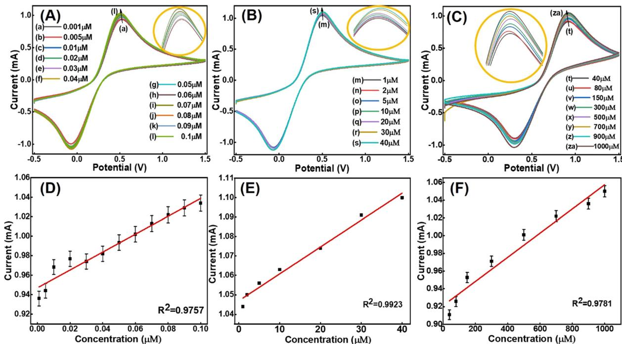
Fig. 7 (A) The CV sensing curve in the concentration range of  $0.001 \text{ }\mu\text{M}$ – $0.1 \text{ }\mu\text{M}$ , (B) the CV curve in the concentration range of  $1 \text{ }\mu\text{M}$ – $40 \text{ }\mu\text{M}$  and (C) the CV sensing curve in the concentration range of  $40 \text{ }\mu\text{M}$ – $1000 \text{ }\mu\text{M}$ , and (D)–(F) plot of the corresponding linear regression coefficients.
