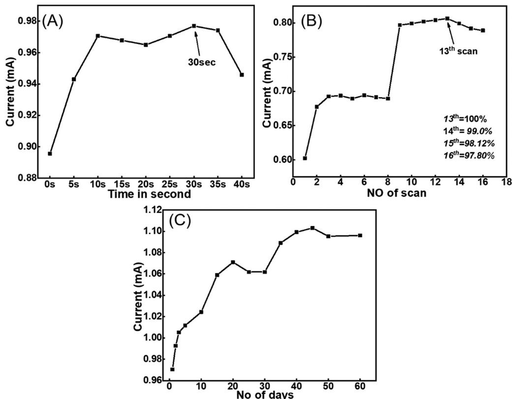
Fig. 9 (A) The response time and (B) the reusability of the prepared Tyr/LaMn<sub>2</sub>O<sub>5</sub>/ITO bioelectrode. (C) The stability graph obtained for the rare phase Tyr/LaMn<sub>2</sub>O<sub>5</sub>/ITO bioelectrode.
