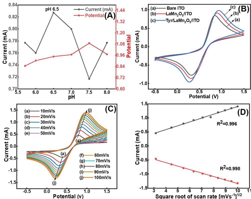
Fig. 6 (A) CV of the pH study for the Tyr/LaMn<sub>2</sub>O<sub>5</sub>/ITO bioelectrode. (B) CV of the bare ITO (a), LaMn<sub>2</sub>O<sub>5</sub>/ITO electrode (b) and Tyr/LaMn<sub>2</sub>O<sub>5</sub>/ITO bioelectrode (c). (C) The scan rate of the Tyr/LaMn<sub>2</sub>O<sub>5</sub>/ITO bioelectrode from 10 to 100 mV s<sup>-1</sup>. (D) Calibration curve of the scan rate study.
