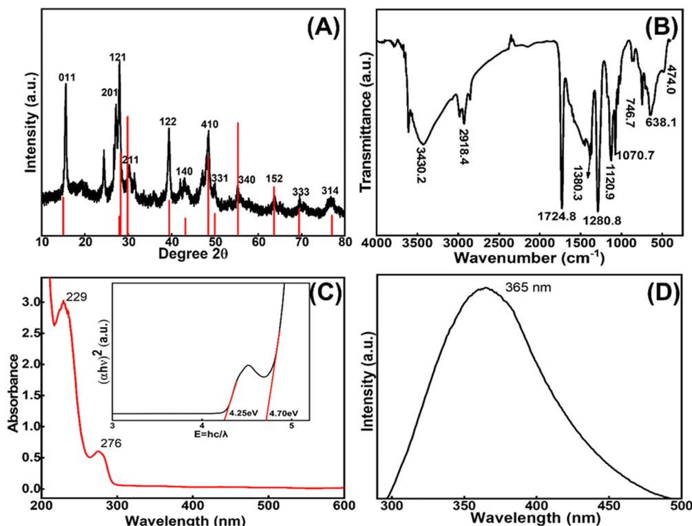
Fig. 2 (A) X-ray diffraction crystallography of  $\text{LaMn}_2\text{O}_5$ , (B) FT-IR spectra of rare phase nanostructure  $\text{LaMn}_2\text{O}_5$ , (C) UV-visible spectra of  $\text{LaMn}_2\text{O}_5$  (inset: the Touc plot of the UV graph representing the binding energy of  $\text{LaMn}_2\text{O}_5$ ) and (D) Photoluminescence spectra of rare phase nanostructure  $\text{LaMn}_2\text{O}_5$ .
