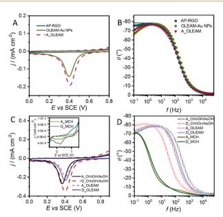
Fig. 5 (A) and (C) CV curves collected at the scan rate of  $0.1 \, \mathrm{V \, s^{-1}}$  and step potential of 0.005 V and (B) and (D) Bode plots at +0.25 V in 0.1 M PBS (pH = 7.4) of SPCEs modified by (A) and (B) AP-RGO, OLEAM-Au NPs and A\_OLEAM, (C) and (D) A\_OLEAM, D\_OLEAM, A\_CH3OH/AcOH, D\_CH3OH/AcOH and (inset of C) A\_MCH and D\_MCH.
