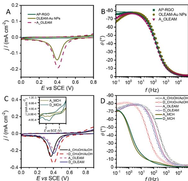
Fig. 5 (A) and (C) CV curves collected at the scan rate of 0.1 V s<sup>-1</sup> and step potential of 0.005 V and (B) and (D) Bode plots at +0.25 V in 0.1 M PBS (pH = 7.4) of SPCEs modified by (A) and (B) AP-RGO, OLEAM-Au NPs and A\_OLEAM, (C) and (D) A\_OLEAM, D\_OLEAM, A\_CH<sub>3</sub>OH/AcOH, D\_CH<sub>3</sub>OH/AcOH and (inset of C) A\_MCH and D\_MCH.
