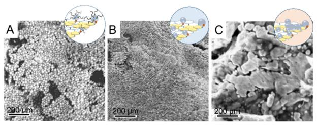
SEM micrographs of SPCEs modified with A\_OLEAM (A), A\_CH<sub>3</sub>OH/AcOH (B) and A\_MCH (C), respectively
