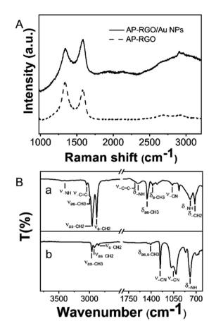
Fig. 3 (A) Raman spectrum of AP-RGO and AP-RGO/Au NPs. (B) FTIR-ATR spectra of neat OLEAM (a) and AP-RGO/Au NPs (b)
