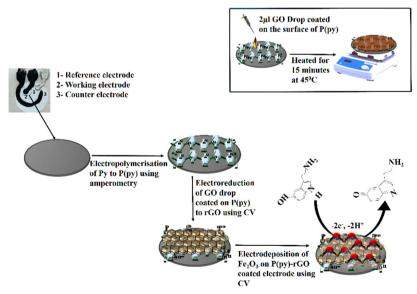
Scheme 1 Schematic illustration of the synthesis of the P(py)-rGO-Fe<sub>2</sub>O<sub>3</sub> ternary nanocomposite on the surface of the PPE, and the inset shows the drop-coating method.
