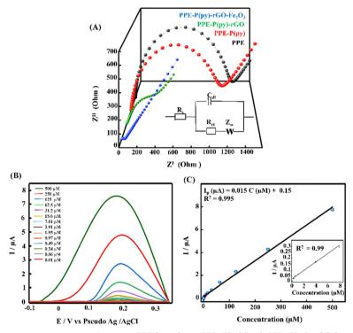
Fig. 5 (A) Electrochemical impedance spectroscopy of the bare PPE (black) and PPE-P(py) (red), PPE-P(py)-rGO (green), and PPE-P(py)-rGO-Fe<sub>2</sub>O<sub>3</sub> (blue) modified electrodes in 0.1 M KCl solution containing 5 mM [Fe(CN)<sub>6</sub>]<sup>3-/4-</sup>. (B) DPV for the different concentrations of 5-HT from 500  $\mu$ M to 0.01  $\mu$ M. (C) The corresponding calibration plot (inset shows the linear calibration plot from 7.81  $\mu$ M to 0.01  $\mu$ M for 5-HT).
