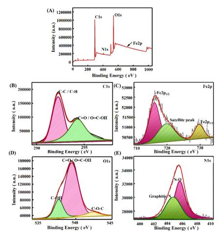
Fig. 3 XPS wide scan deconvoluted spectrum of PPE-P(py)-rGO-Fe<sub>2</sub>O<sub>3</sub>. (A) XPS survey scan. (B) Deconvoluted C1s spectrum. (C) Deconvoluted Fe<sub>2</sub>p spectrum. (D) Deconvoluted O1s spectrum. (E) Deconvoluted N1s spectrum
