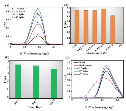
Fig. 6 (A) DPV voltammogram for the recovery study. (B) Histogram showing the selectivity of the developed PPE-P(py)-rGO-Fe<sub>2</sub>O<sub>3</sub> sensor towards interfering species (AA, UA, DA, E). (C) Histogram depicting the results of the stability study conducted on the PPE-P(py)-rGO-Fe<sub>2</sub>O<sub>3</sub> sensor stored at room temperature for a period of 15 days. (D) DPV response for *Drosophila melanogaster* brain samples.
