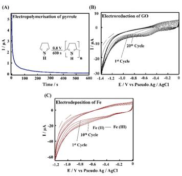
Fig. 1 (A) Amperometry profile of electrodeposition of P(py) in solution containing 0.01 M pyrrole in 0.1 M PB solution (pH 7.4). (B) Cyclic voltammograms of the electro-reduction of 2  $\mu$ L GO drop coated on PPE-P(py). (C) Cyclic voltammograms of the electrodeposition of Fe<sub>2</sub>O<sub>3</sub> on PPE-P(py)-rGO.
