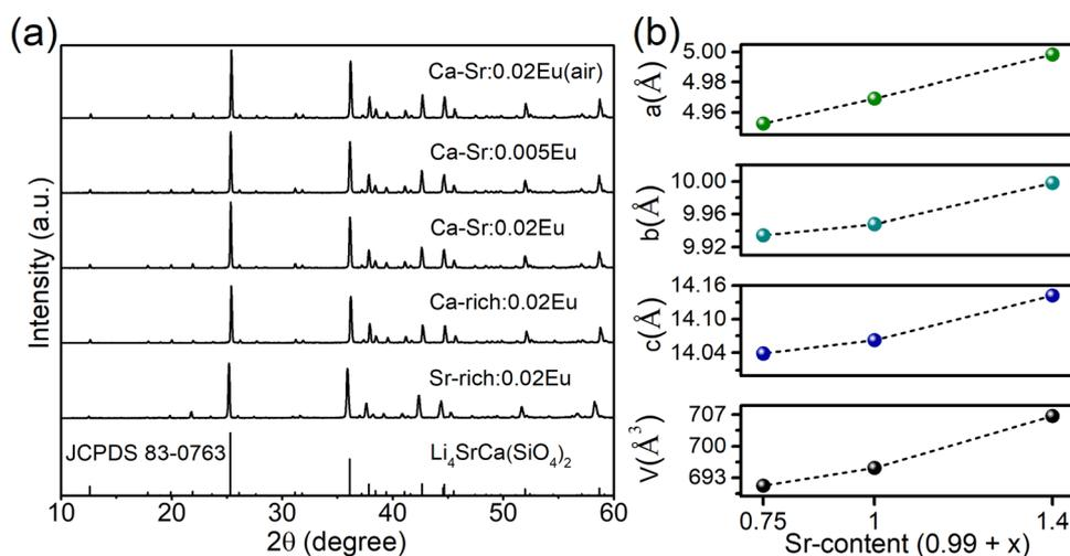
Fig. 1 (a) XRD patterns of all samples and the reference pattern of  $\text{Li}_4\text{SrCa}(\text{SiO}_4)_2$  (JCPDS 83-0763). (b) The lattice parameters extracted from the XRD patterns for the samples prepared under a reducing atmosphere with 0.02Eu concentration.
