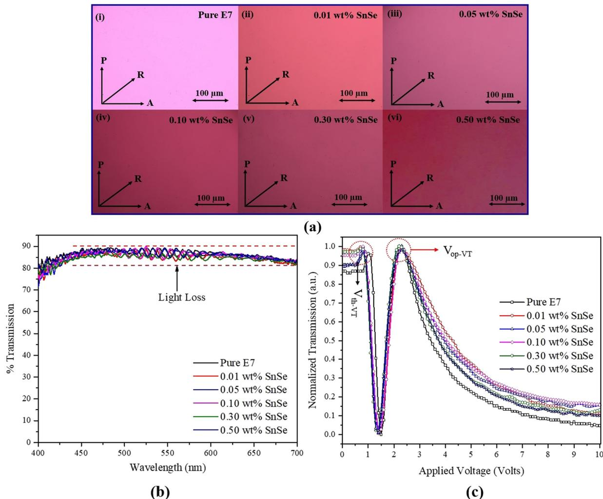
Fig. 2 POM textures in the bright state (a) (P, R and A represents the polarizer, analyser and rubbing direction of LC cells), transmission spectrum (b) and  $V$ - $T$  curve (at  $f = 1$  kHz) (c) of pure E7 and SnSe blended LC cells at RT.
