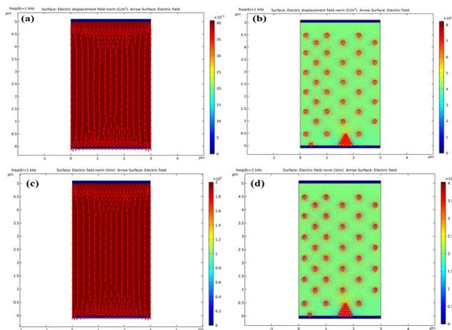
**Fig. 8** Calculated distribution of electric flux density (a and b) and electric field (c and d) of pure E7 and SnSe blended LC Cell respectively. The electric field direction is indicated by the red arrow, while the color represents the field strength.
