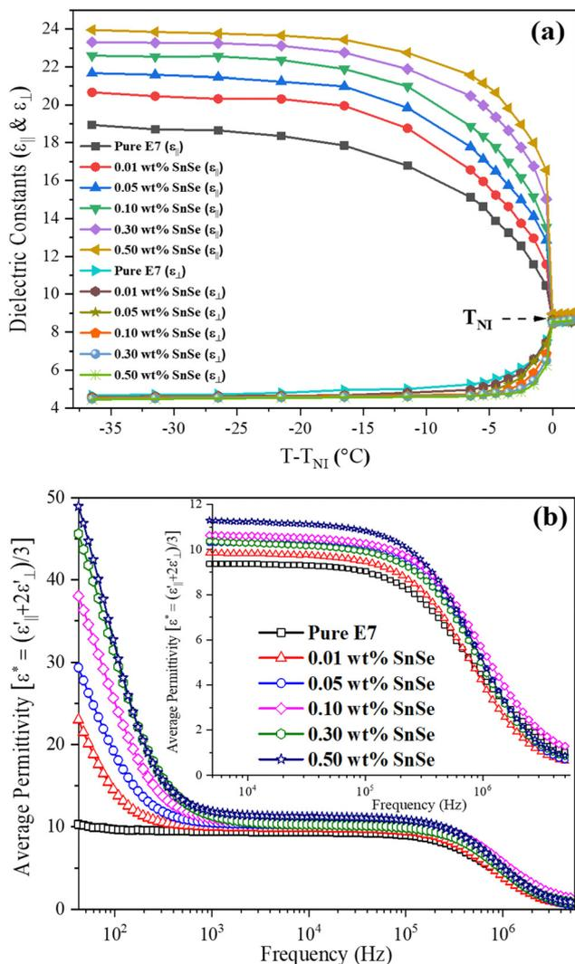
Fig. 4 (a) Variation of parallel and perpendicular components of the dielectric constant (at 1 kHz  $> f_{EP}$ ) with reduced temperature for pure E7 and SnSe-blended LC cells, and (b) the average permittivity of LC cells at room temperature with various concentrations of SnSe nanospheres. The inset of (b) represents an enlarged view of the average permittivity from 5 kHz to 5.5 MHz.
