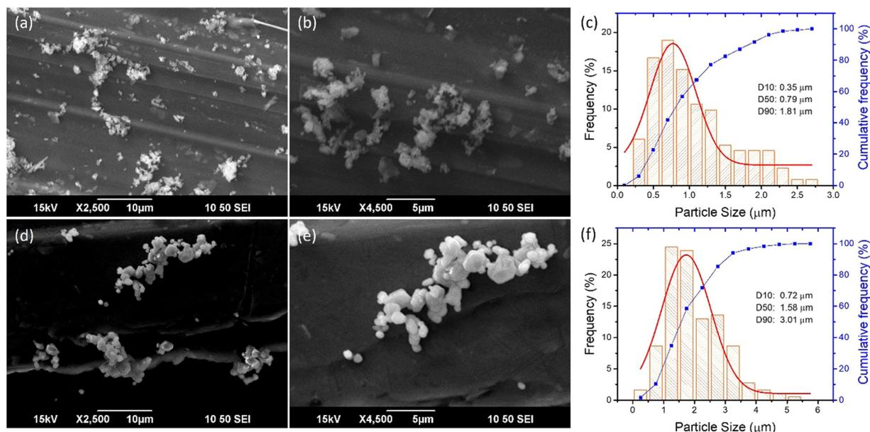
Fig. 5 SEM images of MgO commercial powders (a) and (b) before firing and (d) and (e) after firing at 1000  $^\circ\text{C}$ . Particle size distribution of MgO commercial powders (c) before firing and (f) after firing.
