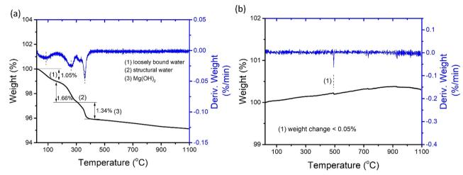
Fig. 6 Temperature-dependent mass recorded for (a) raw MgO powder and (b) MgO powder after firing at 1000 °C
