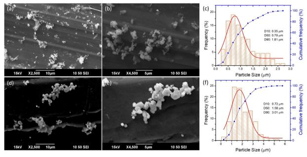
Fig. 5 SEM images of MgO commercial powders (a) and (b) before firing and (d) and (e) after firing at 1000 °C. Particle size distribution of MgO commercial powders (c) before firing and (f) after firing
