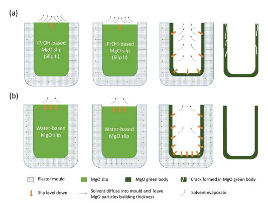
Fig. 4 Schematic diagrams depicting the slip casting processes using (a) an iPrOH-based MgO slip (slip II) and (b) a water-based MgO slip with favourable flowability.
