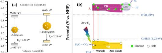
Scheme 2 The band positions of CQD@CdS and N-CQD@CdS photocatalyst (a). The photocatalytic hydrogen generation mechanism (b) for phase engineered, sulfur vacancy enriched, and CQD loaded CdS nanostructures.
