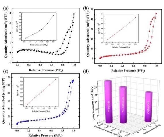
The BET absorption-desorption isotherms (a)-(c), and the pore size distribution and surface area (d) of the CdS sample
