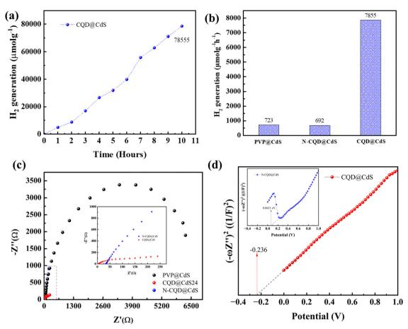
Fig. 7 Hydrogen generation (a) using seawater with CQD@CdS for 10 hours. A comparison of the hydrogen generation rate using seawater (b), EIS spectra (c) and Mott–Schottky plot (d) for all the CdS samples.
