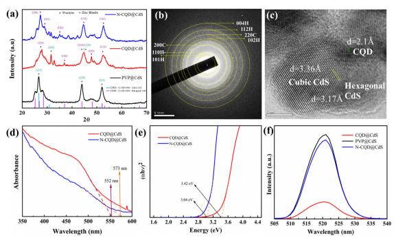
Fig. 1 Shows the diffraction pattern (a), absorbance spectra (d), Tauc plot (e) and photoluminescence spectra (f) of all the CdS samples, and the SAED (b) and TEM lattice fringes (c) of the CQD@CdS samples.
