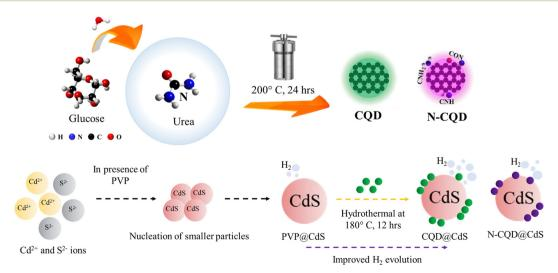
Scheme 1 This shows the synthesis process of carbon quantum dots (CQDs) and the CQD integrated cadmium sulfide photocatalyst.
