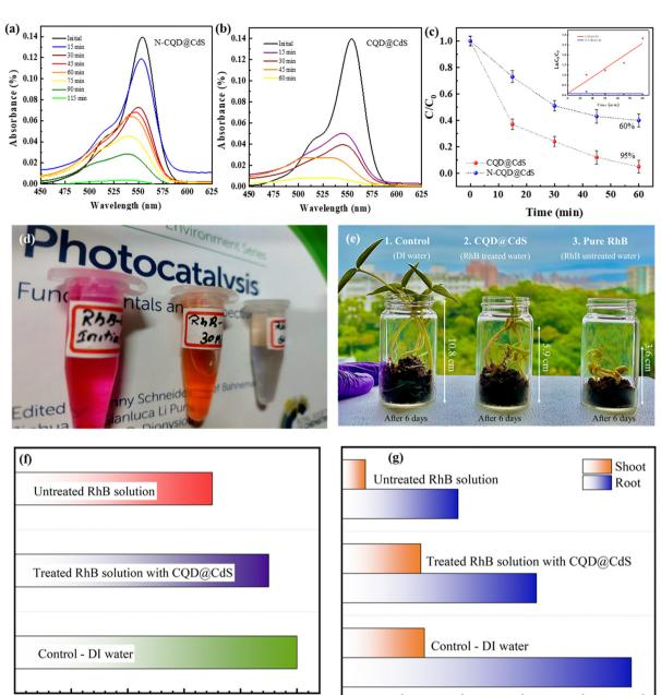
Fig. 5 The Rhodamine B degradation absorbance spectra by N-CQD@CdS (a), and CQD@CdS samples (b). Dye degradation efficiency and pseudosecond order kinetic plot (c), change of dye over a 60 min time period (d), Vigna radiata growth rate profile with different sources of water (e) and growth rate (f), roots and shoots lengths (g).
