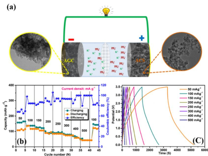
Fig. 8 Electrochemical performance of the AGC//ACS K-ion capacitor: (a) schematic illustration of the fabrication of the KIC full cell, (b) rate capability at current densities from 50 to  $500 \text{ mA g}^{-1}$ , and (c) GCD curves recorded at different current densities.
