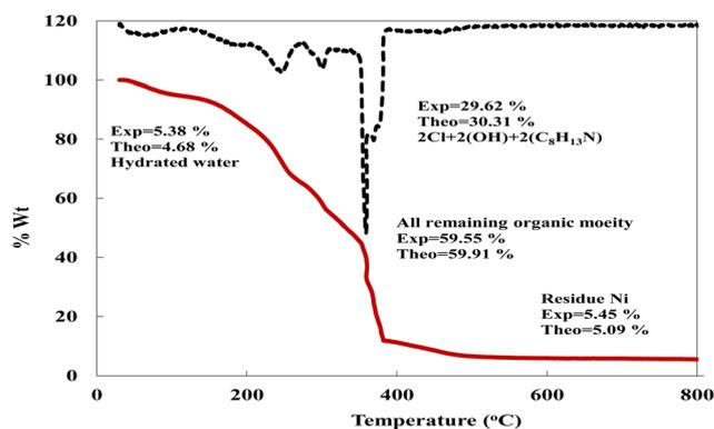
Fig. 3 TG curve of the prepared Ni(II)-SB complex.
