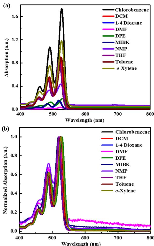
Fig. 3 (a) Absorption spectra with different solvents. (b) Normalized absorption spectra with other solvents.
