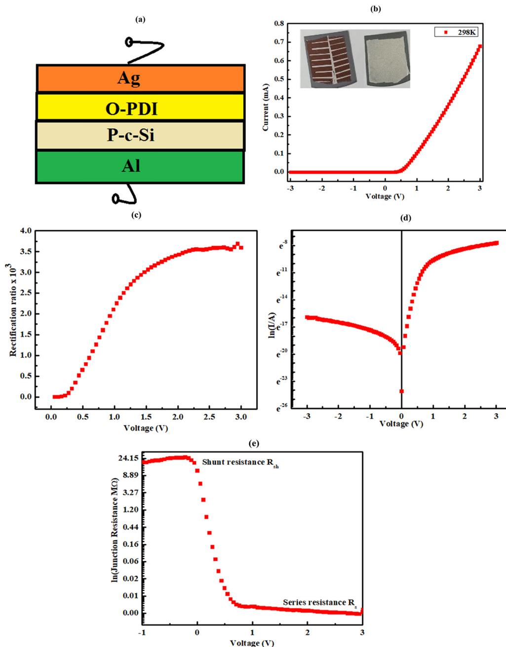
**Fig. 10** Heterojunction device Al/P-c-Si/O-PDI/Ag fabricated using synthesized O-PDI and all the analysis carried out at room temperature under the dark condition, (a) schematic of the heterojunction device, (b) *I-V* characteristics at room temperature and the inset shows the actual device from the back and front side, (c) rectification curve of device, (d) semi-logarithmic (*I-V*) characteristics, and (e) junction resistance vs. voltage.
