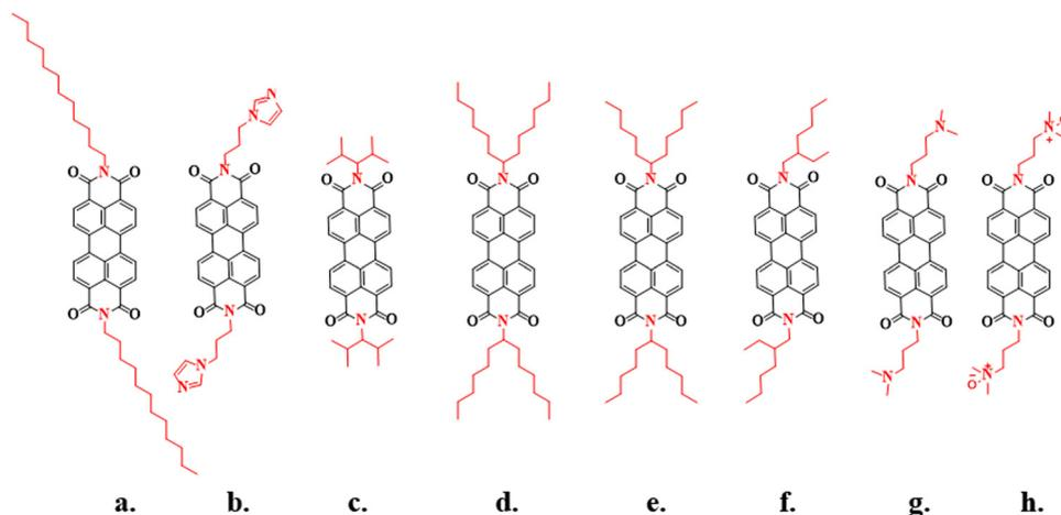
Fig. 1 Previously reported imide substituted PDI small molecules.
