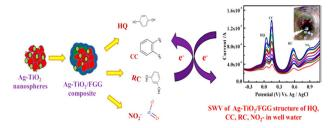
Fig. 13 Schematic representation of Aq-TiO<sub>2</sub>/functionalized guar gum NC for the detection of hydroguinone, catechol, resorcinol, and nitrite (reprinted from ref. 156 with permission from Elsevier).
