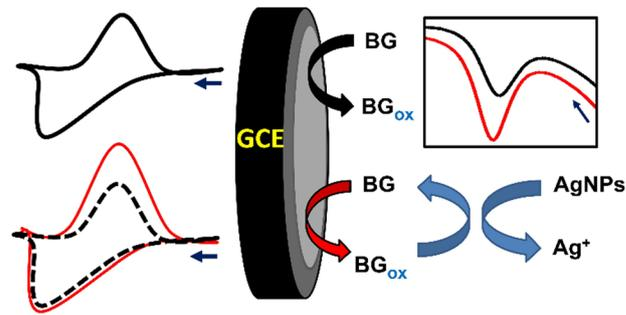
Fig. 2 Schematic representation of the detection of bromocresol green dye using AgNPs as a redox mediator.<sup>54</sup>
