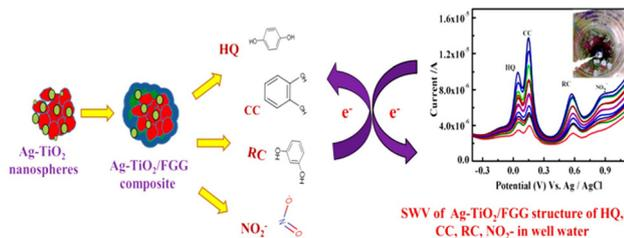
Fig. 13 Schematic representation of Ag–TiO<sub>2</sub>/functionalized guar gum NC for the detection of hydroquinone, catechol, resorcinol, and nitrite (reprinted from ref. 156 with permission from Elsevier).
