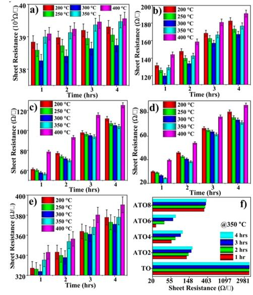
Fig. 7 Thermal stability studies of the (a) TO, (b) ATO2, (c) ATO4, (d) ATO6, and (e) ATO8 thin films at 200-400 °C with different annealing durations of 1, 2, 3, and 4 h. (f) Comparison of the sheet resistance of the films annealed for different durations at 350 °C.
