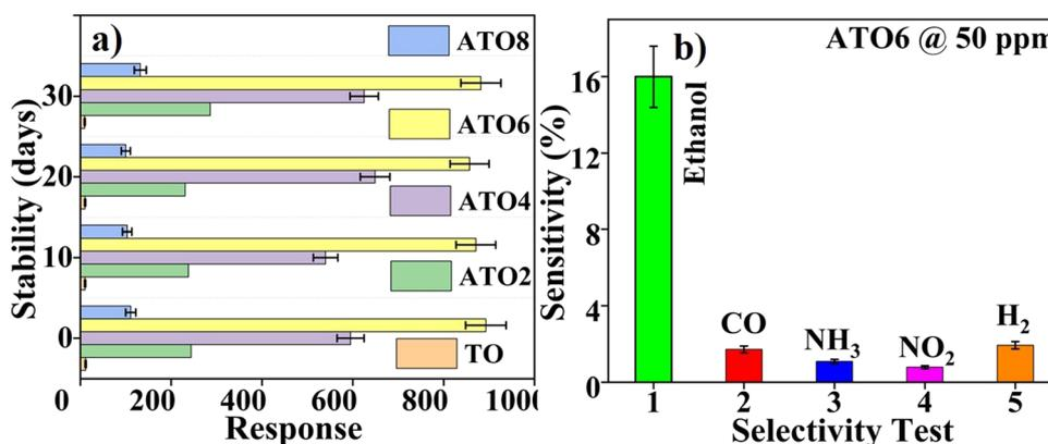
Fig. 10 (a) Stability study of TO and ATO films towards 50 ppm of ethanol gas at 30 °C. (b) Selectivity test of the TO and ATO films towards ethanol, CO, NH<sub>3</sub>, H<sub>2</sub>, and NO<sub>2</sub> gases injected at 50 ppm at 30 °C.
