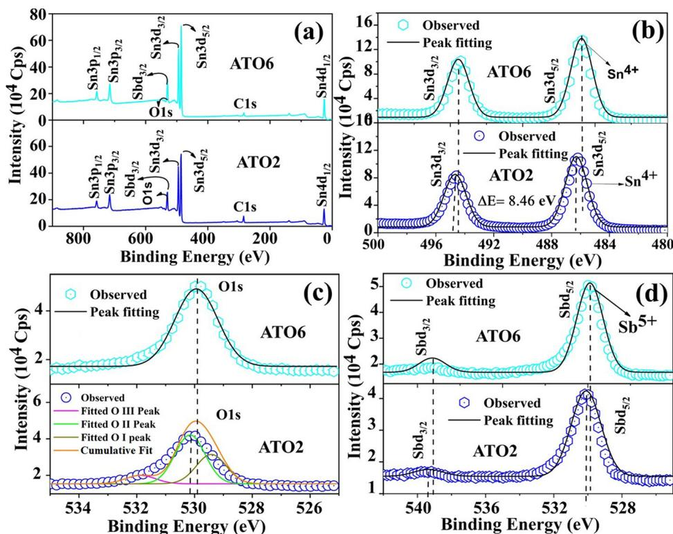
Fig. 6 The XPS full survey scan spectrum (a), Sn3d narrow scan spectrum (b), O1s narrow scan spectrum (c), and Sb3d narrow scan spectra (d) for ATO420 and ATO450 films.
