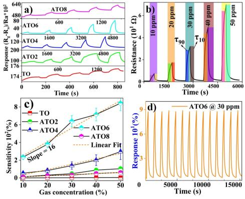
Fig. 8 (a) Gas sensing behavior of the TO and ATO films towards ethanol gas at 10-50 ppm. (b) Enlarged view of the sensing behavior of the ATO6 films. (c) Sensing plot. (d) Cyclic response study of an ATO6 film towards 50 ppm of ethanol.
