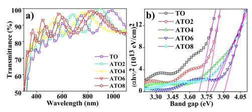
Fig. 5 (a) Transmittance spectra of TO and ATO films with different Sb contents and (b) Tauc plots of the films as a function of the Sb-doping content.
