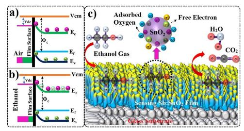
Fig. 9 Schematic of the energy band diagram along with charge transport processes in the presence of air (a) and ethanol (b). Schematic of the ethanol sensing mechanisms of ATO films (c)
