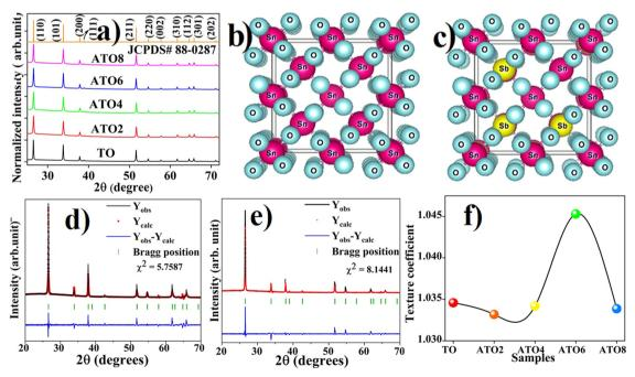
Fig. 1 (a) XRD patterns of TO and ATO films and the standard XRD pattern of SnO2. (b) and (c) Crystal structures of undoped and Sb-doped SnO2 systems. Rietveld refinement XRD patterns of (d) TO and (e) ATO6 films. (f) Texture coefficient (TC<sub>hkl</sub>) of the TO and ATO thin films.
