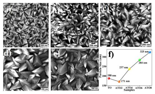
Fig. 2 FE-SEM surface morphology images of the (a) TO, (b) ATO2, (c) ATO4, (d) ATO6, and (e) ATO8 thin films. (f) ImageJ software estimated particle size from FE-SEM mages of the TO and ATO films.
