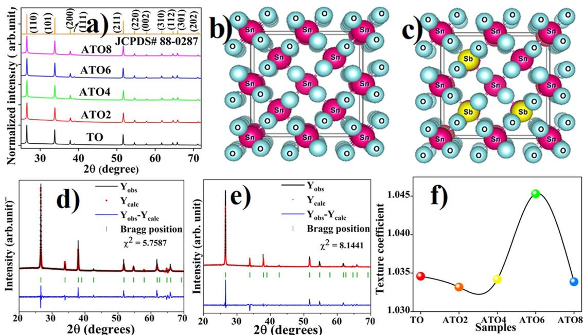
Fig. 1 (a) XRD patterns of TO and ATO films and the standard XRD pattern of  $\text{SnO}_2$ . (b) and (c) Crystal structures of undoped and Sb-doped  $\text{SnO}_2$  systems. Rietveld refinement XRD patterns of (d) TO and (e) ATO6 films. (f) Texture coefficient ( $TC_{hkl}$ ) of the TO and ATO thin films.
