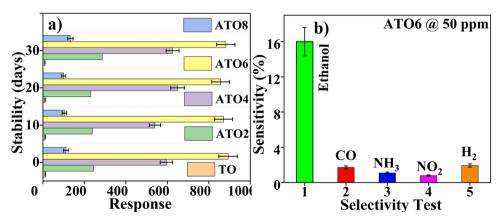
Fig. 10 (a) Stability study of TO and ATO films towards 50 ppm of ethanol gas at 30 °C. (b) Selectivity test of the TO and ATO films towards ethanol, CO, NH<sub>3</sub>, H<sub>2</sub>, and NO<sub>2</sub> gases injected at 50 ppm at 30 °C.
