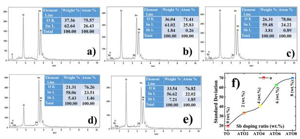
Fig. 3 EDS spectra of the Sn, O, and Sb elemental composition ratio of the films: (a) TO, (b) ATO2, (c) ATO4, (d) ATO6, and (e) ATO8 thin films. (f) The variation of the standard deviation with the Sb doping ratio of the TO and ATO films.
