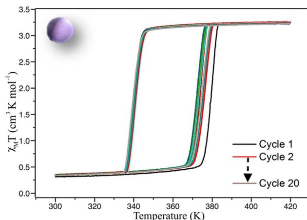
Fig. 5  $\chi_M T$  product versus  $T$  recorded for molecular ceramic of **1** (C1) showing the evolution of the magnetic properties in 20 cycles. Scan rate = 5 K min<sup>-1</sup>.
