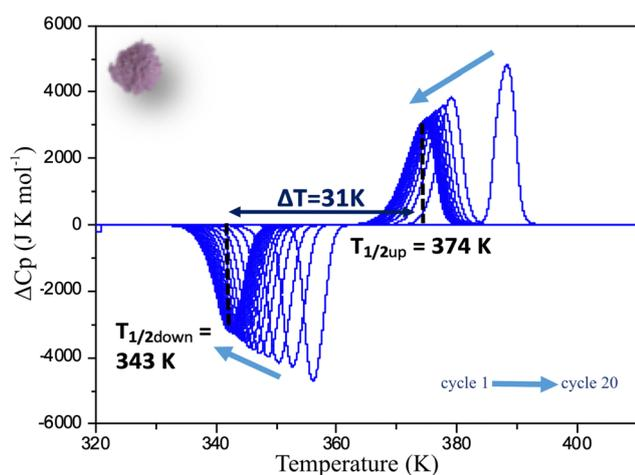
Fig. 3 Deviation from normal molar heat capacity ( $\Delta C_p$ ) vs. temperature for **1** recorded by DSC on a powder sample at  $5 \text{ K min}^{-1}$ . Arrows are showing the evolution from the first to the 20th cycle.  $\Delta C_p$  peaks in the cooling mode are artificially represented negatives, that way, the endothermic process corresponds to a positive peak in the chart.
