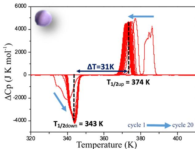
Fig. 6 Deviation from normal molar heat capacity ( $\Delta C_p$ ) vs. temperature for a molecular ceramic of **1** recorded by DSC at  $5 \text{ K min}^{-1}$ . Arrows show the evolution from the first to the 20th cycle.
