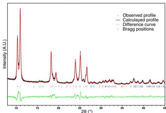
Fig. 4 Rietveld refinement results on powder X-ray diffraction pattern of molecular ceramic of **1** (C1) at 293 K. Experimental pattern (black cross), calculated pattern (red line), Difference curve (green line), Bragg positions (vertical lines).
