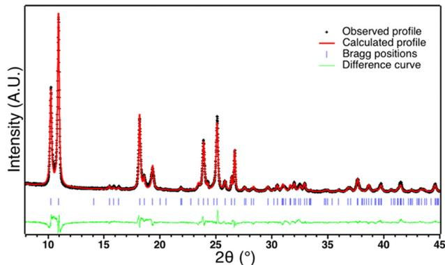
Fig. 1 Rietveld refinement results on powder X-ray diffraction pattern of **1** at 293 K. Experimental pattern (black cross), calculated pattern using polymorph I data (red line), Difference curve (green line), Bragg positions (vertical lines).
