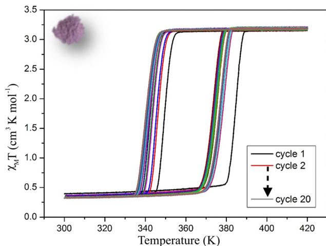
Fig. 2  $\chi_M T$  product versus  $T$  recorded on a powder sample of **1** showing the evolution of the magnetic properties upon 20 cycles. Scan rate =  $5 \text{ K min}^{-1}$ .
