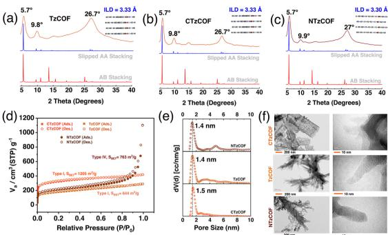
Fig. 1 XRD patterns of (a) TzCOF, (b) CTzCOF, and (c) NTzCOF along with their simulated slipped AA stacking patterns. (d) N2 adsorption isotherms of COFs along with their (e) statistical pore-size distribution (QSDFT method, cylindrical pore, and N2 on carbon at 77 K). (f) TEM images.
