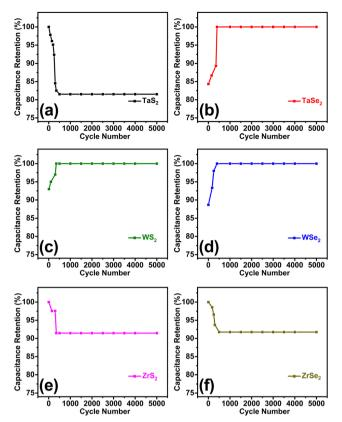
Fig. 5 Stability curves of (a) TaS<sub>2</sub>, (b) TaSe<sub>2</sub>, (c) WS<sub>2</sub>, (d) WSe<sub>2</sub>, (e) ZrS<sub>2</sub> and (f) ZrSe<sub>2</sub> electrodes measured for the first 5000 cycles.
