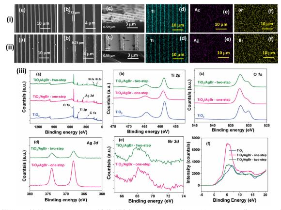
Fig. 6 FE-SEM images (a)-(c) and elemental mapping (d)-(f) of TiO<sub>2</sub>/AgBr nanocomposites fabricated through one-step (i) and two-step (ii) methods. (iii) (a) XPS survey scan of TiO<sub>2</sub>/AgBr nanocomposites in comparison to pristine TiO<sub>2</sub>; XPS narrow scan of (b) Ti 2p, (c) O 1s, (d) Ag 3d and (e) Br 3d of the nanocomposites; (f) overlay of VB spectra of TiO2 and its nanocomposite with AgBr obtained via the two approaches
