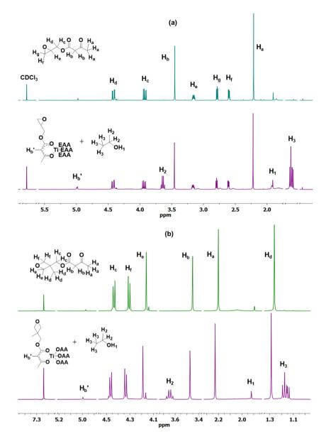
Fig. 1 <sup>1</sup>H NMR spectra of EAA (a) and OAA (b) before and after complexation with titanium(IV) ethoxide to formulate Ti(EAA)<sub>4</sub> and Ti(OAA)<sub>4</sub> resins. The respective chemical structures shown in the inset are labelled for indicating the characteristic peaks.
