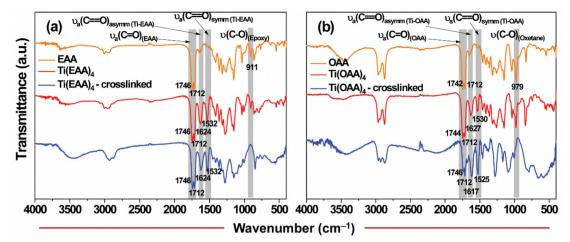
Fig. 2 Probing of metal chelation and ring opening polymerization in (a) Ti(EAA)4 and (b) Ti(OAA)4 resin formulations through FT-IR analyses
