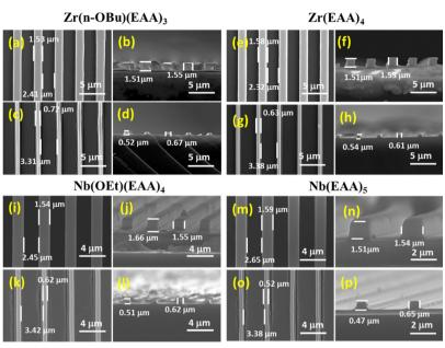
Fig. 5 Aerial and cross-sectional FE-SEM images of the imprints obtained using resin formulations of Zr(n-OBu)(EAA)<sub>3</sub> (a)-(d), Zr(EAA)<sub>4</sub> (e)-(h), Nb(OEt)(EAA)<sub>4</sub> (i)-(l) and Nb (EAA)<sub>5</sub> (m)-(p). The top and bottom lanes in each panel represent imprints before and after calcination, respectively.
