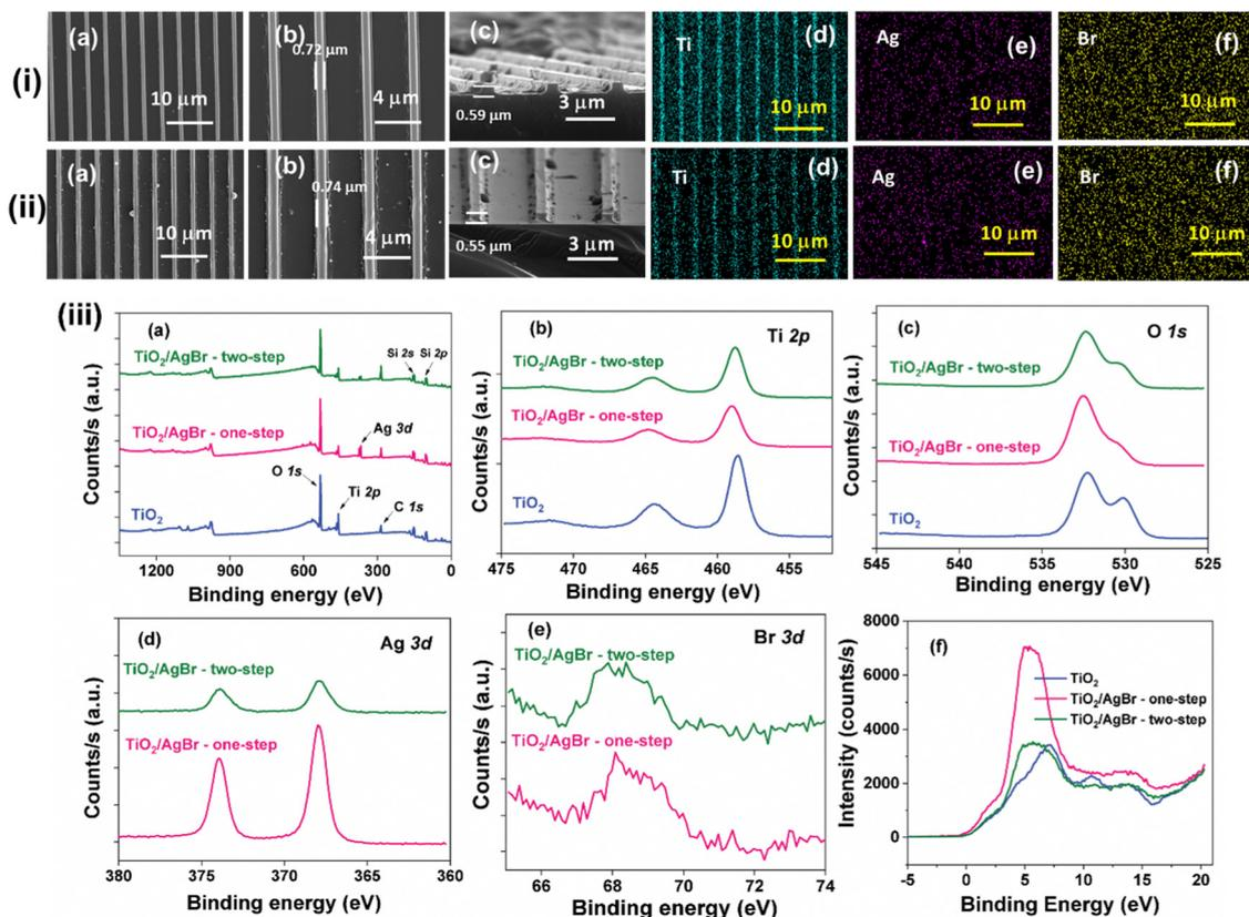
**Fig. 6** FE-SEM images (a)–(c) and elemental mapping (d)–(f) of TiO<sub>2</sub>/AgBr nanocomposites fabricated through one-step (i) and two-step (ii) methods. (iii) (a) XPS survey scan of TiO<sub>2</sub>/AgBr nanocomposites in comparison to pristine TiO<sub>2</sub>; XPS narrow scan of (b) Ti 2p, (c) O 1s, (d) Ag 3d and (e) Br 3d of the nanocomposites; (f) overlay of VB spectra of TiO<sub>2</sub> and its nanocomposite with AgBr obtained *via* the two approaches.
