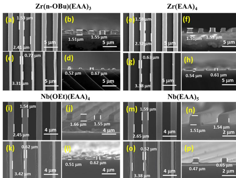
Fig. 5 Aerial and cross-sectional FE-SEM images of the imprints obtained using resin formulations of  $\text{Zr}(n\text{-OBu})(\text{EAA})_3$  (a)–(d),  $\text{Zr}(\text{EAA})_4$  (e)–(h),  $\text{Nb}(\text{OEt})(\text{EAA})_4$  (i)–(l) and  $\text{Nb}(\text{EAA})_5$  (m)–(p). The top and bottom lanes in each panel represent imprints before and after calcination, respectively.
