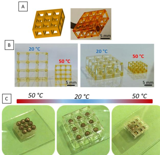
Fig. 5 (A) STL file of the "bead trap" and picture of the fabricated device by SLA just after printing with PiPrOx<sub>20</sub>-*net*-PAM<sub>4</sub>. (B) View of the volume shrinking above the VPTT for PiPrOx<sub>20</sub>-*net*-PAM<sub>4</sub>. (C) Proof of concept of the "bead trap" design below and above the VPTT using the hydrogel PMOx<sub>20</sub>-*net*-PNIPAM<sub>100</sub>.
