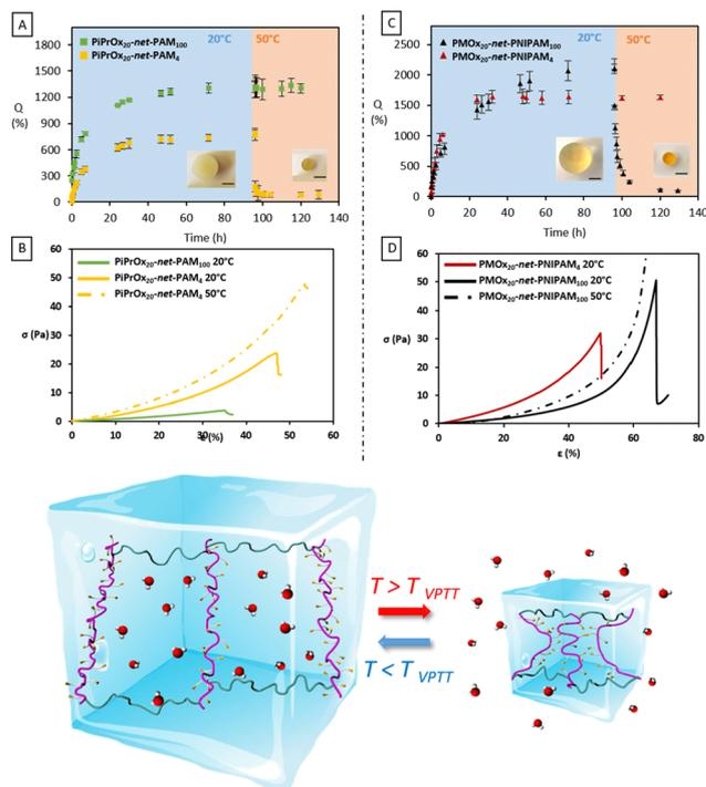
Fig. 4 Swelling kinetics in water at 20 and 50 °C and compressing tests of (A) and (B) PMOx<sub>20</sub>-net-PNIPAM<sub>100</sub> and PMOx<sub>20</sub>-net-PNIPAM<sub>4</sub> and (C) and (D) PiPrOx<sub>20</sub>-net-PAM<sub>100</sub> and PiPrOx<sub>20</sub>-net-PAM<sub>4</sub> (scale bar 5 mm).
