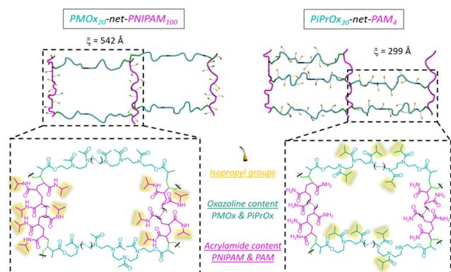
Fig. 2 Synthesis of the hydrogels based on copolymers  $PMOx_{20}$ -*net*-PNIPAM<sub>100</sub> (5/1) and  $PiPrOx_{20}$ -*net*-PAM<sub>4</sub> (5/1), and illustration of the resulting networks. Blue corresponds to POx blocks, purple for acrylamide units and green for methacrylate moieties.
