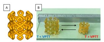
Fig. 6 (A) CAD model of a porous cylindrical stent. (B) Picture of the printed devices by SLA using PiPrOx<sub>20</sub>-net-PAM<sub>4</sub> copolymer and showing the contraction of the stent device above and under the VPTT.
