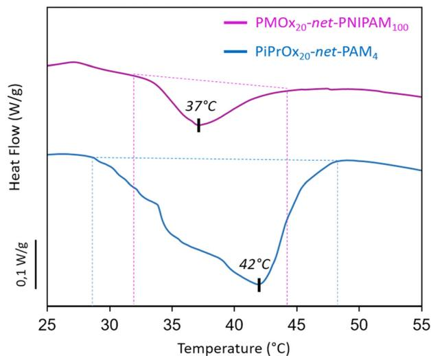
Fig. 3 Thermogram of hydrogels PiPrOx<sub>20</sub>-net-PAM<sub>4</sub> and PMOx<sub>20</sub>-net-PNIPAM<sub>100</sub> by using DSC (5 °C min<sup>-1</sup>).
