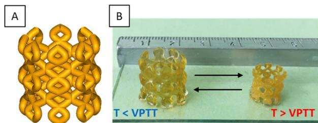
Fig. 6 (A) CAD model of a porous cylindrical stent. (B) Picture of the printed devices by SLA using PiPrOx<sub>20</sub>-*net*-PAM<sub>4</sub> copolymer and showing the contraction of the stent device above and under the VPTT.
