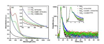
Fig. 11 Working electrodes of CS1, CS2 and CS3 along with a TiO<sub>2</sub> reference electrode for (a) UV-vis absorption and (b) electron lifetime analysis; (inset) expanded x-axis scale.
