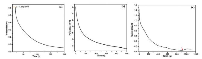
Fig. 10 Time-dependent analysis of CS1 (a) OCVD with 10 s of light illumination; (b) OCVD under dark condition; (c) current under dark and IR-free
