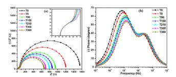
Fig. 7 Device exposed to LED lamp at 40 mW cm $^{-2}$ . (a) Impedance analysis at various time intervals; (inset) expanded initial region. (b) Bode plot derived from impedance analysis.
