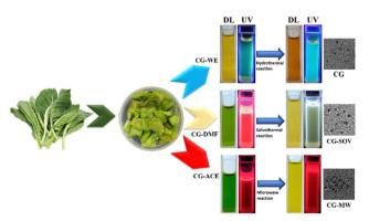
Fig. 1 A schematic representation of the collard green CD synthesis. CG-WE stands for collard greens extract in water and ethanol solvent, CG-DMF stands for collard greens extract in DMF solvent and CG-ACE stands for collard greens extract in acetone solvent while CG, CG-SOV, and CG-MW are their corresponding CDs prepared by hydrothermal, solvothermal and microwave methods, respectively. DL: daylight; UV: ultra-violet light.
