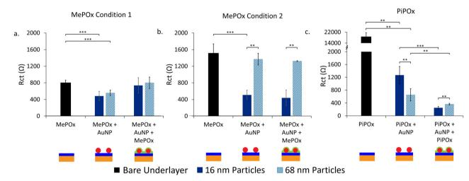
Fig. 3 Fitted R<sub>ct</sub> values for each stage of the sandwich construction with (a) MePOx condition 1, (b) MePOx condition 2, and (c) PiPOx as underlayers. \*\* represents p < 0.01, \*\*\* represents p < 0.001. Schemes beneath give a graphical representation of each stage of layered construction.
