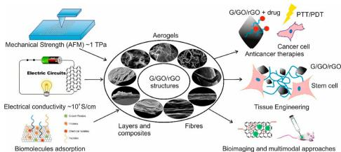
Fig. 6 Schematic showing versatile functionalities of graphene (G), graphene oxide (GO), and reduced graphene oxide (rGO) structures and their typical uses in biomedical devices and systems.<sup>68</sup>
