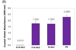
Fig. 8 (A) Images of O-Si-DLC, F-Si-DLC, Si-DLC, and PS with fungal pathogen Candida albicans after crystal violet staining. (B) Crystal violet quantification of C. albicans on O-Si-DLC, F-Si-DLC, Si-DLC, and PS samples using absorbance measured at 600 nm. (O - oxygen, F - fluorine, PS – polystyrene).<sup>130</sup>
