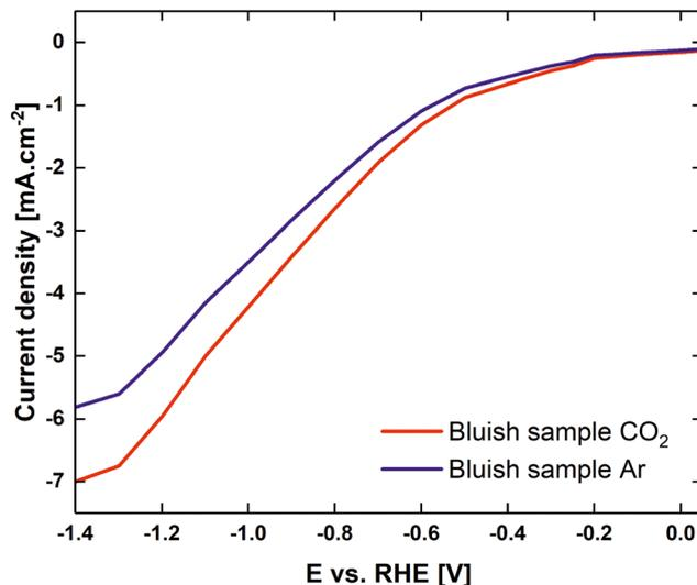
Fig. 6 Linear sweep voltammograms of a  $\text{CO}_2$  purged 0.1 M  $\text{K}_2\text{CO}_3$  electrolyte (red) to pH 6.79, Ar purged 0.1 M  $\text{K}_2\text{CO}_3$  electrolyte (blue) for the bluish sample.
