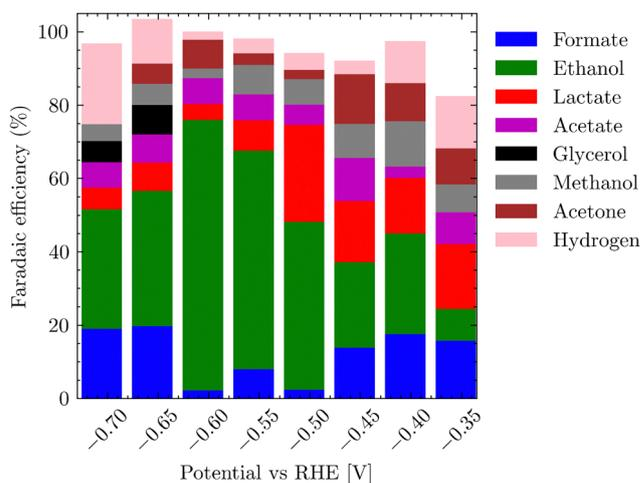
Fig. 7 Dependence of product formation on an applied potential vs. RHE for bluish sample.
