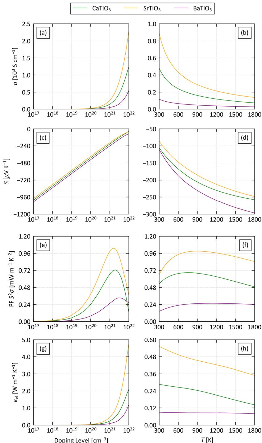
Fig. 4 Comparison of the calculated averaged electrical conductivity  $\sigma$  (a)/(b), Seebeck coefficient  $S$  (c)/(d) power factor  $S^2\sigma$  (PF) (e)/(f) and electronic thermal conductivity  $\kappa_{\text{el}}$  (g)/(h) of the three structures examined in this work as a function of doping level at a fixed  $T = 1000$  K (a)/(c)/(e)/(g) and as a function of temperature at a fixed doping level  $n = 10^{21}$  cm<sup>-3</sup> (b)/(d)/(f)/(h).
