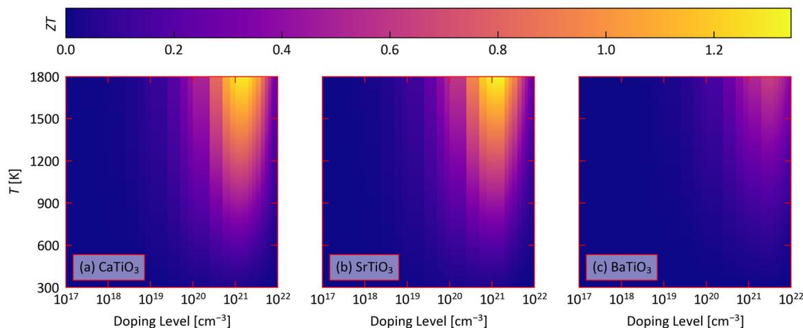
Fig. 5 Predicted thermoelectric figure of merit  $ZT$  of  $\text{CaTiO}_3$  (a),  $\text{SrTiO}_3$  (b) and  $\text{BaTiO}_3$  (c) as a function of doping level  $n$  and temperature obtained using eqn (1).
