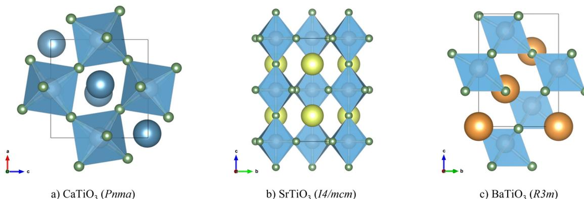
Fig. 1 Conventional cells of  $\text{CaTiO}_3$  in the  $Pnma$  space group (a),  $\text{SrTiO}_3$  in the  $I4/mcm$  space group (b) and  $\text{BaTiO}_3$  in the  $R3m$  space group (c). Atom colours: Ca – blue; Sr – yellow; Ba – orange; Ti – grey; O – green. These images were prepared using the VESTA software.<sup>38</sup>
