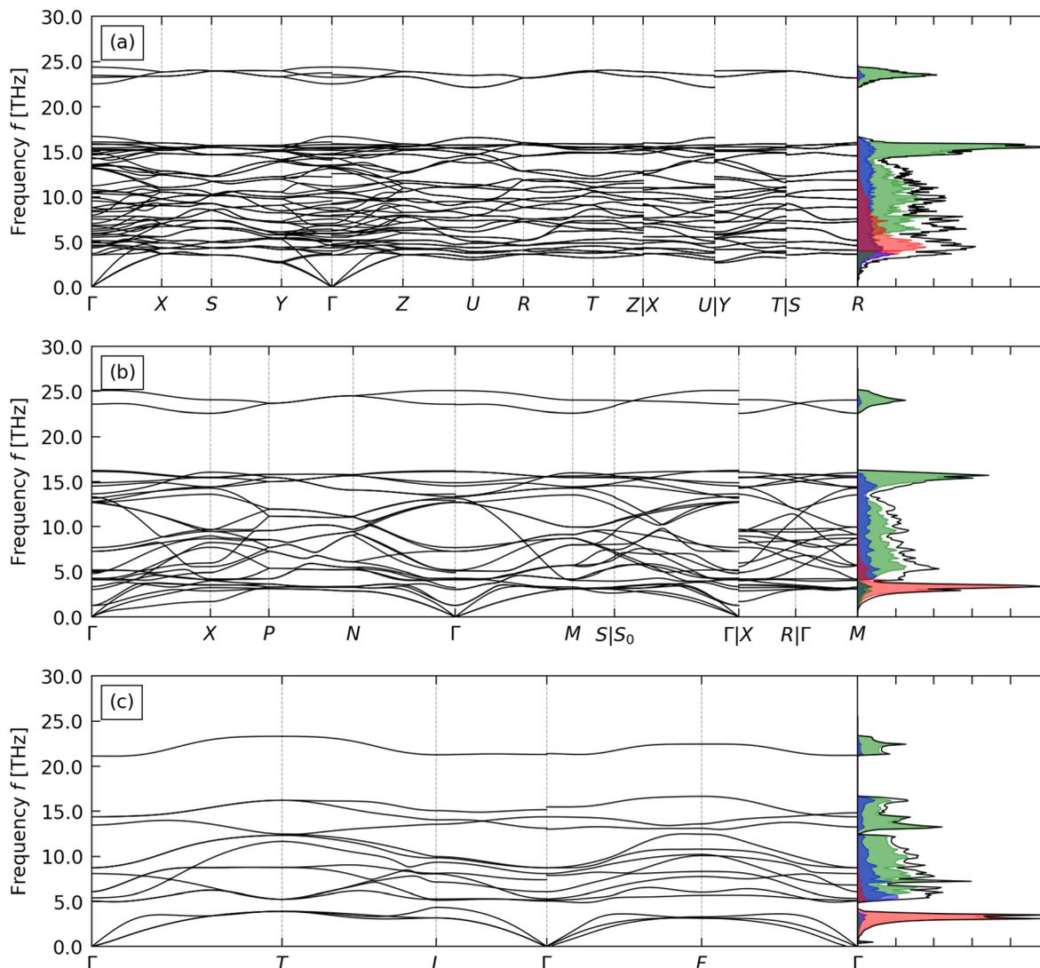
Fig. 2 Calculated phonon dispersion and density of states (DoS) curves of CaTiO<sub>3</sub> (a), SrTiO<sub>3</sub> (b), and BaTiO<sub>3</sub> (c). On each DoS plot, the total DoS is shown in black, and projections onto the A-site cation, Ti and O atoms are shown in red, blue, and green respectively.
