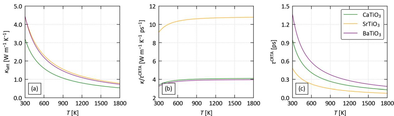
Fig. 3 Analysis of the predicted lattice thermal conductivity of CaTiO<sub>3</sub>, SrTiO<sub>3</sub> and BaTiO<sub>3</sub> using the constant relaxation-time approximation defined in eqn (2): averaged thermal conductivity  $\kappa_{\text{latt}}$  (a), harmonic term  $\kappa/\tau^{\text{CRTA}}$  (b) and averaged lifetime  $\tau^{\text{CRTA}}$  (c) as a function of temperature.
