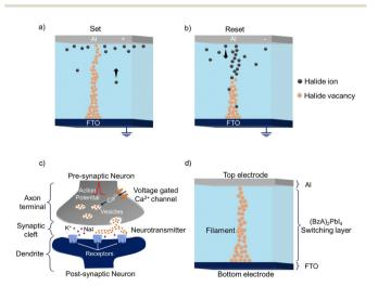
Fig. 4 Resistive switching mechanism in layered hybrid perovskites. Schematic of (a) set (LRS) and (b) reset (HRS) switching governed by ion migration. Illustration of a (c) biological snapse and (d) (BzA)<sub>2</sub>PbI<sub>4</sub>-based artificial synapse mimicking the biological function.
