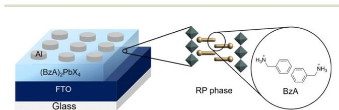
**Fig. 1** Layered hybrid perovskite resistive switching device. Schematic of a resistive switching device architecture (left) based on Ruddlesden–Popper (RP) layered perovskite phase as active material (right) comprising benzylammonium (BzA) cations between aluminium (Al) contacts and fluorine-doped tin oxide (FTO) conductive glass used in this study.
