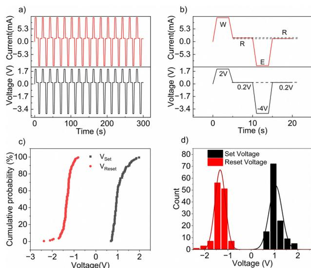
**Fig. 3** Bromide-based perovskite memory data storage and retrieval. (a) Write-read-erase-read (WRER) cycles. (b) Enlarged view of 1st WRER cycle indicating write (W), read (R), and erase (E) states with the corresponding voltage bias. (c) Cumulative probability for set and reset voltages based on 125 cycles. (d) Statistical distribution of set and reset voltages with Gaussian fitted curve. WRER cycles for the iodide-based system are detailed in Fig. S6 of the ESI<sup>†</sup>.
