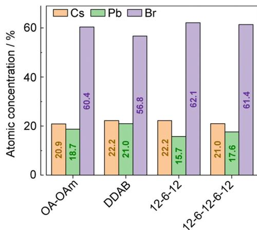
Fig. 4 Atomic concentrations of CsPbBr<sub>3</sub> NCs estimated from the peak areas of the HAXPES narrow scans weighted with sensitivity factors.
