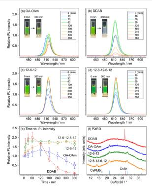
Fig. 2 Results of the water resistance tests: photoluminescence spectra of CsPbBr<sub>3</sub> NCs/(a) OA-OAm, (b) DDAB, (c) 12-6-12, and (d) 12-6-12-6-12 during water exposure. (e) Changes in the relative luminescence intensity of CsPbBr<sub>3</sub> NCs, and (f) XRD patterns of the supernatants obtained after water exposure for 360 min. The light-blue and dark red patterns show the simulated profiles of CsPbBr3 and CsBr, respectively
