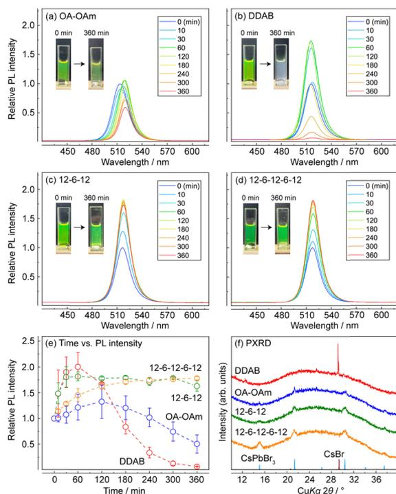
**Fig. 2** Results of the water resistance tests: photoluminescence spectra of CsPbBr<sub>3</sub> NCs/(a) OA–OAm, (b) DDAB, (c) 12-6-12, and (d) 12-6-12-6-12 during water exposure. (e) Changes in the relative luminescence intensity of CsPbBr<sub>3</sub> NCs, and (f) XRD patterns of the supernatants obtained after water exposure for 360 min. The light-blue and dark red patterns show the simulated profiles of CsPbBr<sub>3</sub> and CsBr, respectively.
