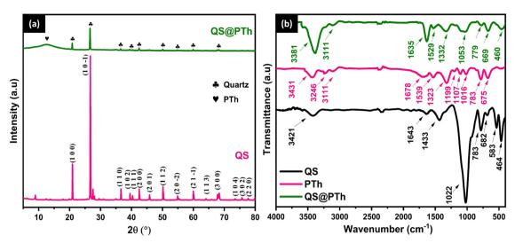
Fig. 1 The X-ray diffraction pattern of QS and QS@PTh (a), and the Fourier-transform infrared spectra of QS, PTh, and QS@PTh (b).
