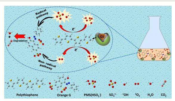
Fig. 6 The proposed mechanism of OG degradation in the QS@PTh/PMS system.
