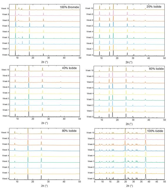
Fig. 4 10 week stability study of thin-films through X-ray diffraction. Graph headings correspond to the proportion of iodide or bromide in the sample.
