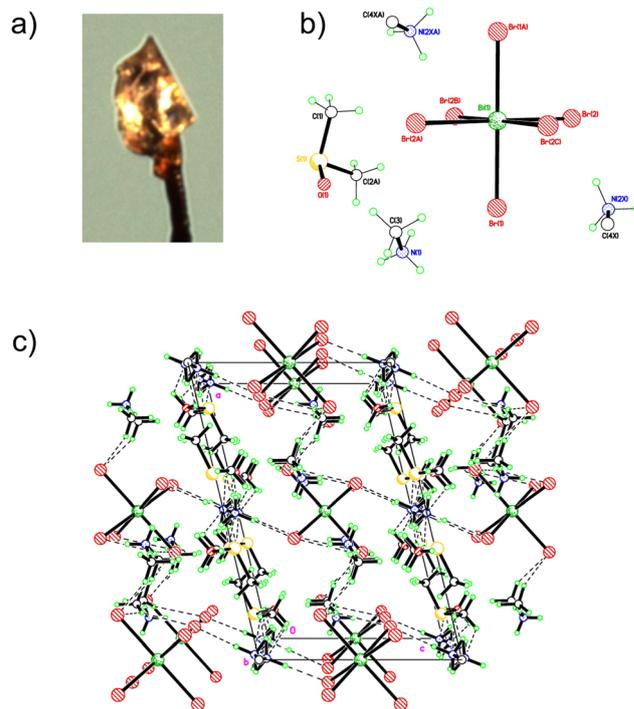
Fig. 1 (a) Photograph of the crystal fragment used for the single crystal X-ray diffraction study, (b) The formula unit in the crystal structure of **1**, with minor DMSO and methyl ammonium disorder components omitted for clarity and (c) Packing plot for **1** showing the extensive H-bonded network of interactions between cations, anions and the DMSO of crystallisation. Structure viewed parallel to *b*.
