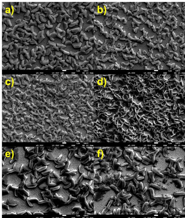
Fig. 5 SEM Images at 5000x magnification of methylammonium bismuth halide films: (a)  $\text{MA}_3\text{Bi}_2\text{I}_9$ , (b)  $\text{MA}_3\text{Bi}_2(\text{I}_{0.8}\text{Br}_{0.2})_9$ , (c)  $\text{MA}_3\text{Bi}_2(\text{I}_{0.6}\text{Br}_{0.4})_9$ , (d)  $\text{MA}_3\text{Bi}_2(\text{I}_{0.4}\text{Br}_{0.6})_9$ , (e)  $\text{MA}_3\text{Bi}_2(\text{I}_{0.2}\text{Br}_{0.8})_9$ , and (f)  $\text{MA}_3\text{BiBr}_6$ .
