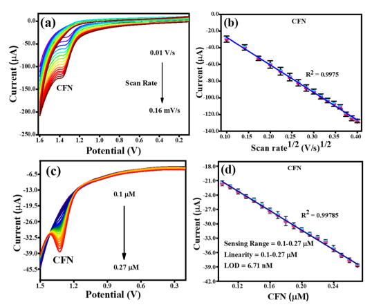
Fig. 7 CV and DPV response for the oxidation of CFN. (a) Effect of CV scan rate on the oxidation of CFN. (b) Dependence of CFN oxidation current on scan rate<sup>1/2</sup>. (c) DPV response for CFN oxidation with increasing concentration. (d) Dependence of oxidation current on CFN concentration
