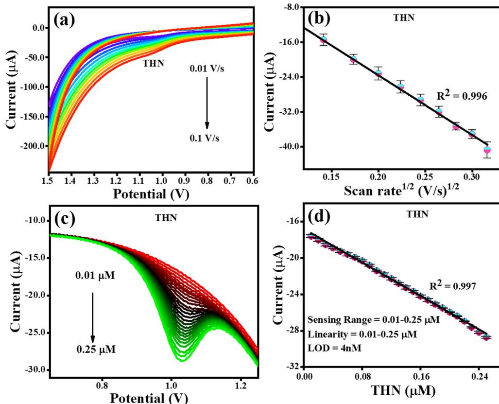
Fig. 8 CV and DPV responses for THN oxidation. (a) Effect of CV scan rate on the oxidation of THN. (b) Dependence of THN oxidation current on scan rate<sup>1/2</sup>. (c) DPV response for THN oxidation reaction with an increase in concentration. (d) Dependence of oxidation current on THN concentration.
