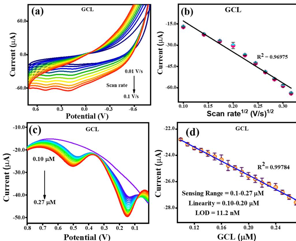
**Fig. 9** CV and DPV response for GCL oxidation. (a) Effect of CV scan rate on the oxidation of GCL. (b) Related GCL oxidation current dependence on scan rate<sup>1/2</sup>. (c) GCL oxidation DPV response with an increase in concentration. (d) Dependence of oxidation current on GCL concentration.
