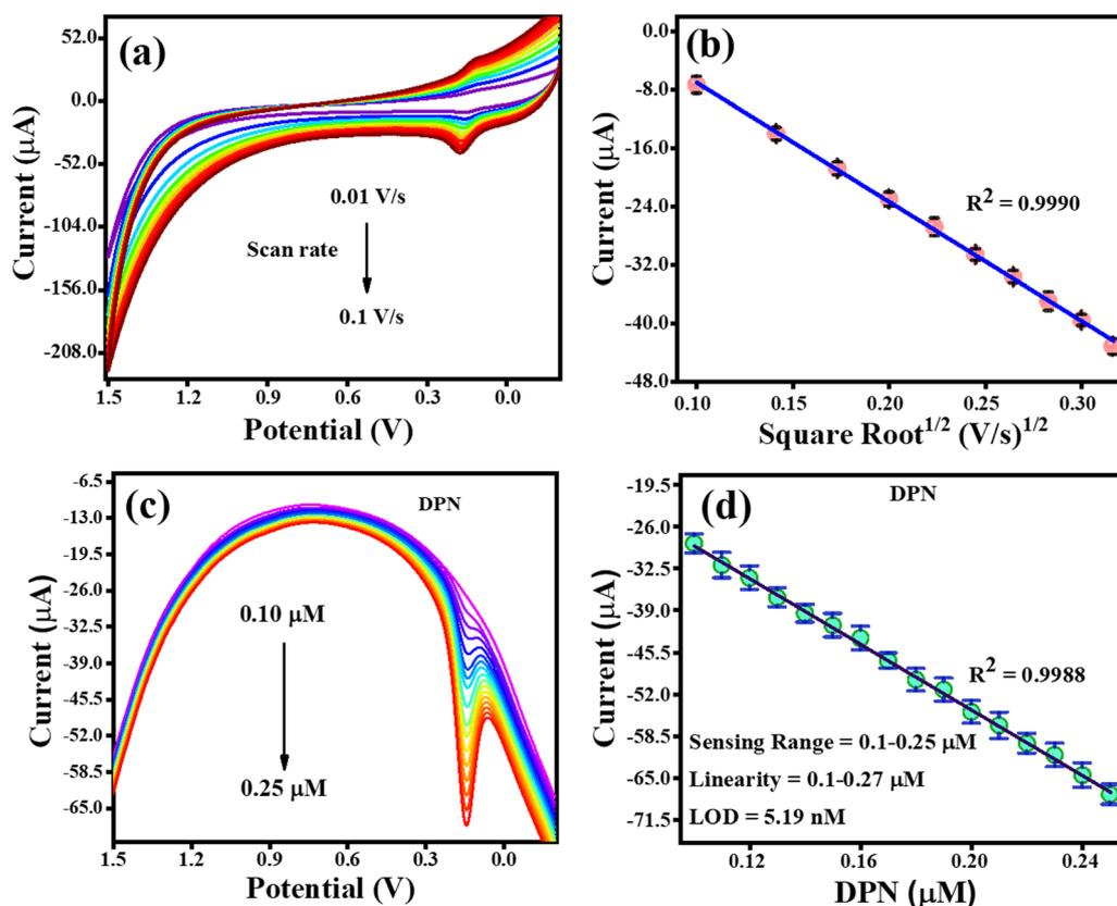
Fig. 10 CV and DPV response for DPN oxidation. (a) Effect of CV scan rate on the oxidation of DPN. (b) Dependence of DPN oxidation current on scan rate<sup>1/2</sup>. (c) DPV response with an increase in the concentration of DPN. (d) Relay oxidation current dependence on DPN concentration.
