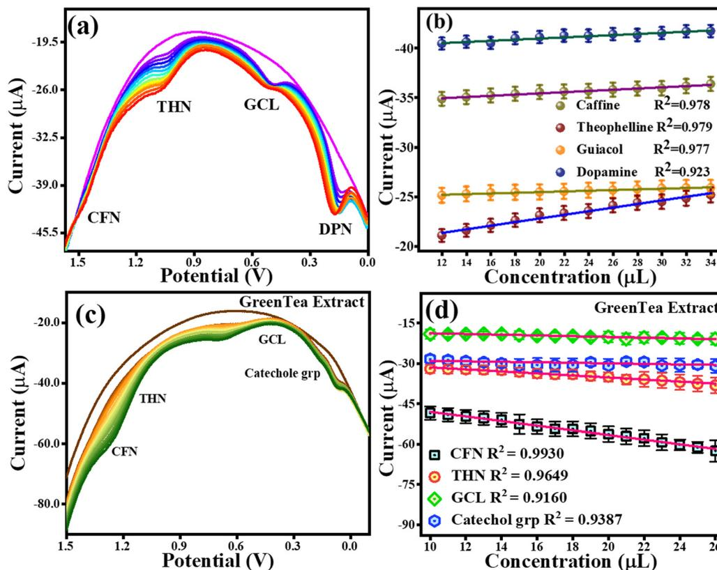
Fig. 11 DPV and CV responses for the oxidation of CFN, THN, GCL and DPN. (a) Effect of DPV scan rate on CFN, THN, GCL and DPN oxidation. (b) Related DPV calibration graph for CFN, THN, GCL and DPN oxidation. (c) DPV response for CFN, THN, GCL and catechol group oxidation with increasing concentration of green tea extract. (d) Dependence of oxidation currents on CFN, THN, GCL and the catechol group.
