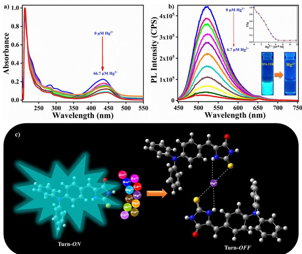
Fig. 5 Change in (a) absorbance and (b) emission spectra of TPA-2TH (3  $\mu\text{M}$ ) upon the addition of different concentrations of Hg<sup>2+</sup> in THF. The inset shows the changes in  $I/I_0$  of TPA-2TH (3  $\mu\text{M}$ ) with increasing concentrations of Hg<sup>2+</sup> (0–6.7  $\mu\text{M}$ ). (c) Pictorial representation of Hg<sup>2+</sup> sensing by TPA-2TH.
