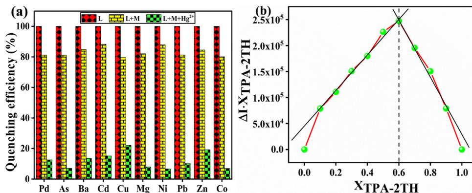
Fig. 6 (a) Interference effect of various metal ions on the emission intensity of TPA-2TH at 522 nm in THF. (b) Job's plot for complex formation between TPA-2TH and Hg<sup>2+</sup> in THF/H<sub>2</sub>O ( $\lambda_{\text{ex}} = 430 \text{ nm}$ ).
