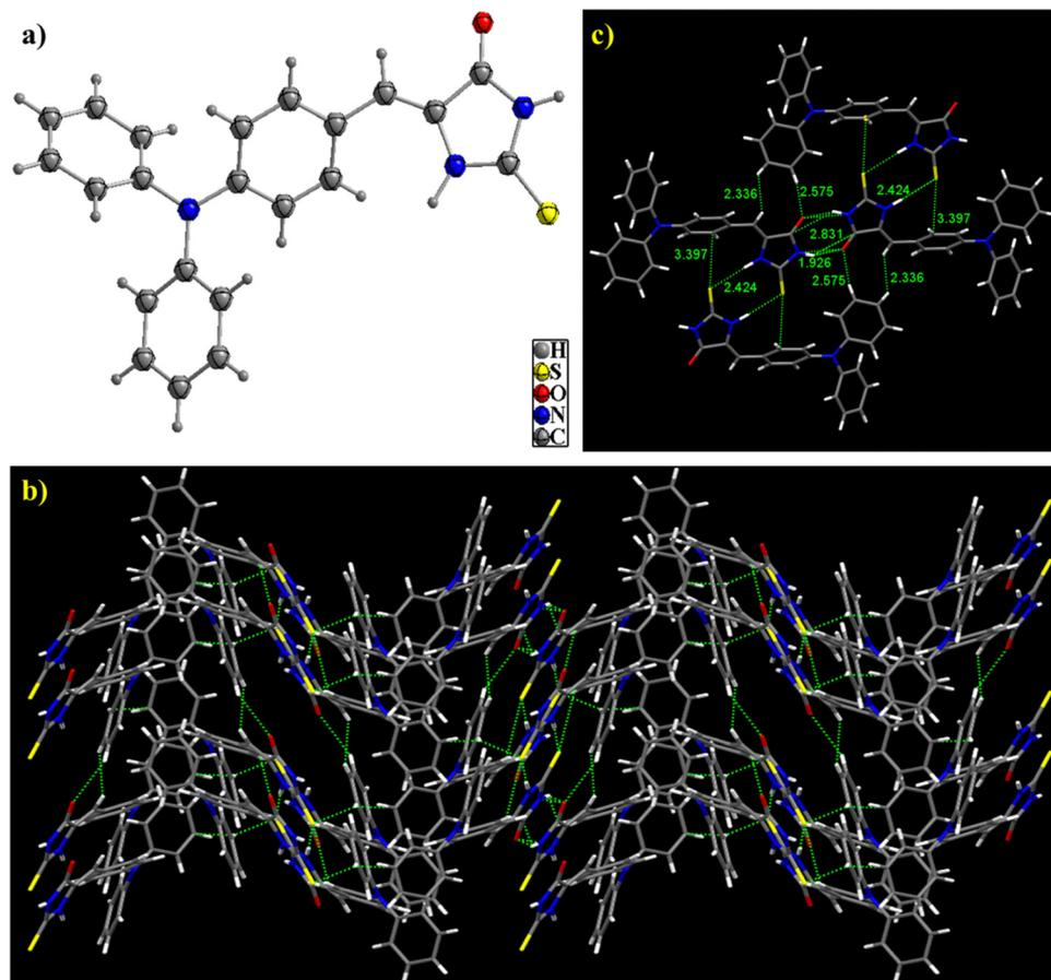
**Fig. 1** (a) Single crystal X-ray structure of **TPA-2TH** with 30% of the thermal ellipsoids. (b) Supramolecular arrangement of **TPA-2TH** in a crystal lattice. (c) Depiction of the crystal packing of the dimeric hydrogen bonding with N–H...S, N–H...O and C–H...O hydrogen bonds followed by C–H... $\pi$  intramolecular interactions.
