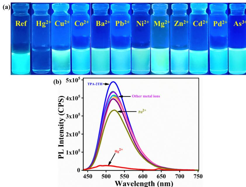
Fig. 4 (a) Photographs of TPA-2TH in the presence of different metal solutions under the UV light of 365 nm. (b) Emission spectra of TPA-2TH (3  $\mu\text{M}$ ) in the absence and presence of different metal ions (6.7  $\mu\text{M}$ ) in THF.
