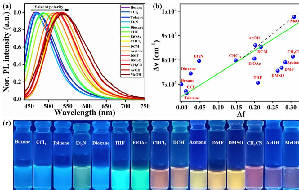
Fig. 3 (a) Emission spectra of TPA-2TH ( $\lambda_{\text{exc}} = 431$  nm) in different solvents, (b) Lippert–Mataga plot in different solvents showing the dependence of the Stokes shift ( $\Delta\nu$ ) of TPA-2TH on the solvent polarity function  $\Delta f$  and (c) photographs showing the changes in emission of TPA-2TH in different solvents under the illumination of UV light (365 nm).
