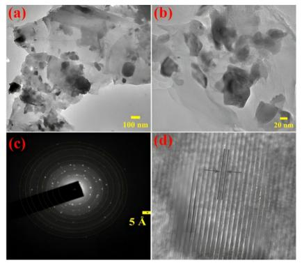
Fig. 2 (a) and (b) TEM pictures of the  $nLa_2O_3$  NPs@rGO composite depicting the rGO sheet-like structure in high and low magnification; (c) SAED pattern; and (d) HR-TEM picture of the  $nLa_2O_3$  NPs@rGO nanocomposite depicting the (222) crystal plane of  $nLa_2O_3$  NPs.
