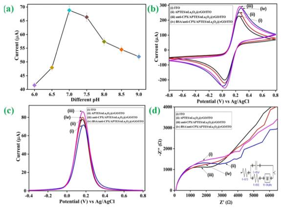
Fig. 5 (a) pH effect of BSA/anti-CPX/APTES/nLa $_2O_3$  NPs@rGO/ITO immunoelectrode; (b) CV; (c) DPV; and (d) EIS study of ITO (curve i), APTES/nLa $_2O_3$  NPs@rGO/ITO (curve iii) and BSA/anti-CPX/APTES/nLa $_2O_3$  NPs@rGO/ITO (curve iv) electrodes [inset depicts the Nyquist circuit diagram].
