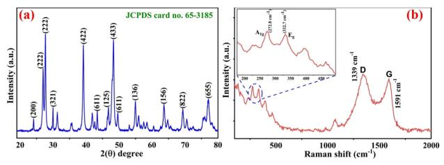
Fig. 1 (a) XRD spectrum; and (b) Raman curve of the nLa<sub>2</sub>O<sub>3</sub> NPs@rGO composite.
