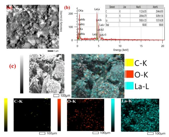
Fig. 3 (a) SEM pictures; (b) EDX spectrum; and (c) elemental mapping of the nLa<sub>2</sub>O<sub>3</sub> NPs@rGO composite.
