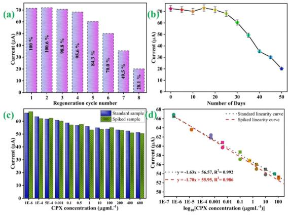
Fig. 9 (a) Regeneration effect studies of the BSA/anti-CPX/APTES/nLa<sub>2</sub>O<sub>3</sub> NPs@rGO/ITO immunosensing platform at a particular concentration of CPX; (b) stability of the developed BSA/anti-CPX/APTES/nLa<sub>2</sub>O<sub>3</sub> NPs@rGO/ITO immunosensor; (c) real spiked milk sample studies versus CPX concentration; and (d) comparative calibration curve in spiked milk and standard samples.
