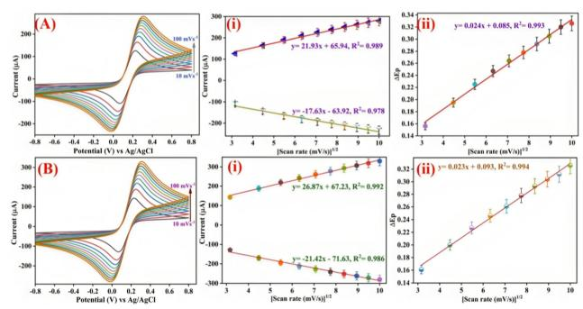
Fig. 6 CV of the (A) APTES/nLa<sub>2</sub>O<sub>3</sub> NPs@rGO/ITO electrode; and (B) BSA/anti-CPX/APTES/nLa<sub>2</sub>O<sub>3</sub> NPs@rGO/ITO immunoelectrode at various scan rates ranging from 10 to 100 mV s<sup>-1</sup>, (A(i)) and (B(i)) calibration curve showing cathodic and anodic current versus square root of scan rate, (A(ii)) and (B(ii)) potential difference ( $\Delta E_p = E_{pa} - E_{pc}$ ) versus square root of the scan rate.
