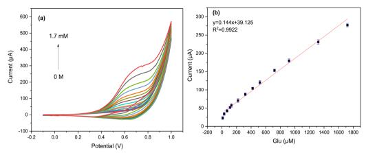
Fig. 7 (a) CVs of Cs/Cu-MOF modified SPCE for different concentrations of glucose (0-1.7 mM) in 0.05 M KOH at a scan rate of 50 mV s<sup>-1</sup>; (b) the correspondence plots of anodic peak currents vs. glucose concentration.
