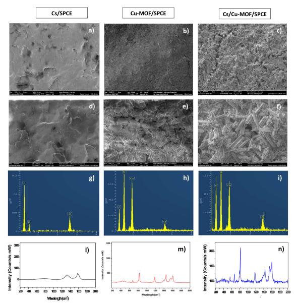
Fig. 4 (a)–(c) SEM images of Cs/SPCE, Cu-MOF/SPCE, and Cs/Cu-MOF taken at low magnification (10  $\mu$ m), respectively; (d)–(f) SEM images of Cs/SPCE, Cu-MOF/SPCE, and Cs/Cu-MOF taken at high magnification (1  $\mu$ m), respectively; (g)–(i) EDX analyses; and (l)–(n) Raman spectra.
