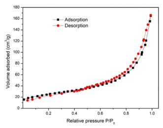
Fig. 3 N<sub>2</sub> adsorption/desorption isotherms of Cu-MOFs.
