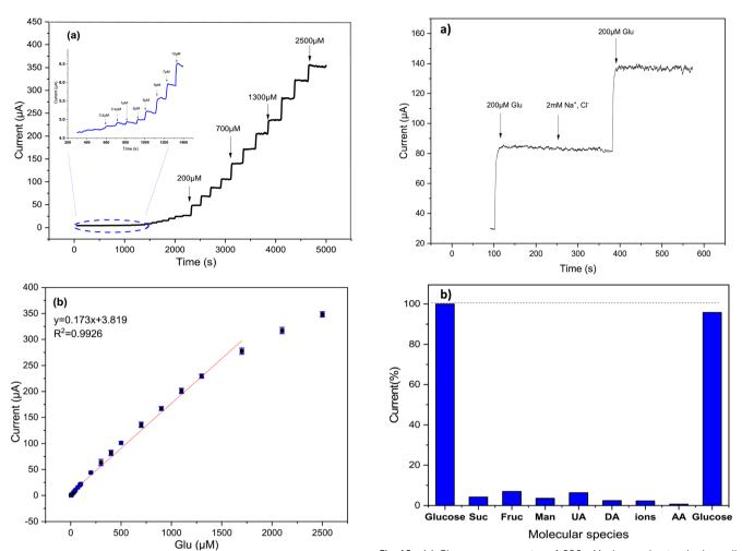
Fig. 9 (a) Amperometric current-time curve of the electrodes of Cs/Cu-MOF/SPCE upon the successive addition of glucose vs. Ag/AgCl holding at 0.7 V in 0.05 M KOH; (b) corresponding calibration curve of current vs glucose concentration.
