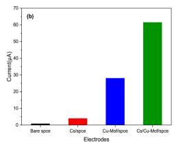
Fig. 6 (a) CVs of the bare SPCE, Cs/SPCE, Cu-MOF/SPCE and Cs/Cu-MOF/SPCE in 0.05 M KOH containing 200 μM glucose at scan rate 50 mV s<sup>-1</sup>. (b) Comparison of the current oxidation peak of glucose at different sensors.
