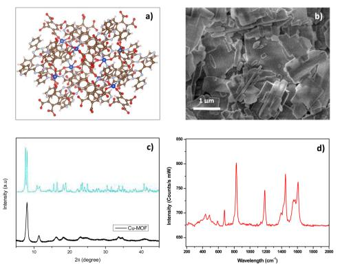
Fig. 1 (a) Possible structure of Cu-MOF by VESTA software (Cu: blue, C: brown, O: sky blue, H: red); (b) SEM mage of Cu-MOF; (c) XRD pattern of Cu-MOF (black curve) compared to pattern (blue curve) described in ref. 42. (d) Raman spectrum of Cu-MOF.
