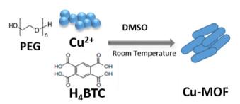
Scheme 1 Preparation process of Cu-MOF.
