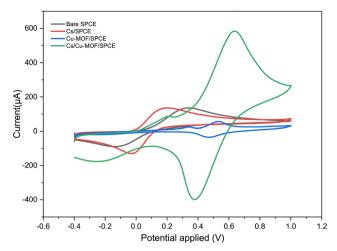
Fig. 5 CVs of Cs/SPCE, Cu-MOF/SPCE, Cs/Cu-MOF/SPCE and bare electrodes in 5 mM  $\rm K_3[Fe(CN)_6]$  and 0.1 M KCl.
