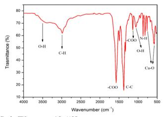
Fig. 2 FTIR spectrum of Cu-MOF.
