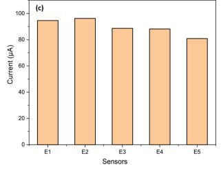
Fig. 11 (a) Repeatability study after successive addition of  $100~\mu M$  glucose by same electrode, (b) stability during 14 days, and (c) reproducibility of 5 Cs/Cu-MOF sensor measurements in 0.05 M KOH.
