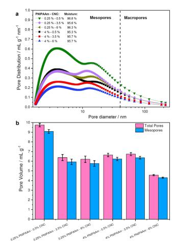
Fig. 5 Quantification of hydrogel porosity. (a) Pore size distribution and (b) pore volume of 0.25 wt% and 4 wt% PNIPAAm-based hydrogels containing 0.5, 3.5, or 6% CNC
