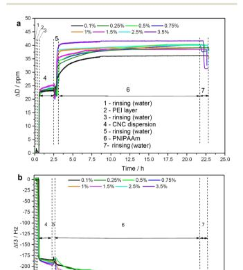
Fig. 1 Quantification of interaction between PNIPAAm and CNC using QCM-D method for hydrogels made from 0.1-3.5 wt% PNIPAAm and 0.5 wt% CNC. (a) Dissipation and (b) Frequency. The numbers mean: 1 rinsing using DI water; 2 - PEI layer deposition; 3 - rinsing; 4 - CNCs layer deposition; 5 - rinsing; 6 - PNIPAAm layer deposition; 7 - rinsing.
