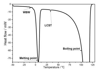
DSC thermogram of 1 wt% PNIPAAm-3.5 wt% CNC hydrogel.
