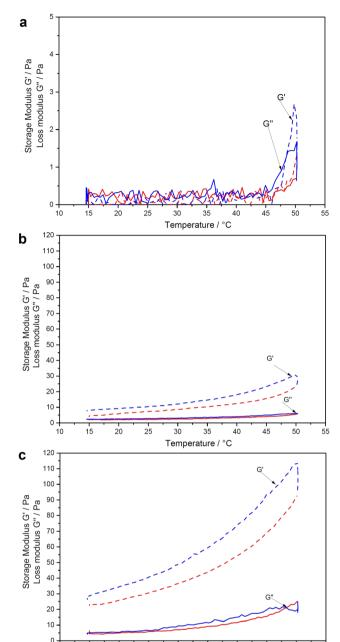
Fig. 4 Rheological analysis of PNIPAAm-CNC hydrogels represented as storage modulus (G') and loss modulus (G'') of hydrogels made within 24 hours from 0.25 wt% PNIPAAm and (a) 0.5 wt%, (b) 3.5 wt%, and (c) 6 wt% CNC. Frequency sweeps were performed at 1% strain and 0.8 rad s<sup>-1</sup> strain.
