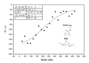
Fig. 2 Isothermal titration calorimetry to study the thermodynamic characteristics of the interaction between CNC and PNIPAAm. Integral plot obtained performing subsequent injections of 10 µL PNIPAAm 3.8 wt% to 0.5 wt% CNC, and fit according to the Levenberg-Marquardt algorithm. Chemical structures of the compounds of interest and values obtained by ITC for the adsorption of PNIPAAm on CNCs
