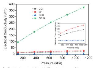
Fig. 3 Electrical conductivities of different carbons and the commercial grade graphene powder with compression. Data represent the average value of 3 repeated experiments, whose results vary less than 3%. Inset: Magnified view of electrical conductivity plots for the biocarbon produced from waste burlap at 600 °C (BC6), commercial graphene (CG) and carbon black (SP). The extremely high conductivity of GB12 is due to the presence of highly graphitized carbons in the sample.
