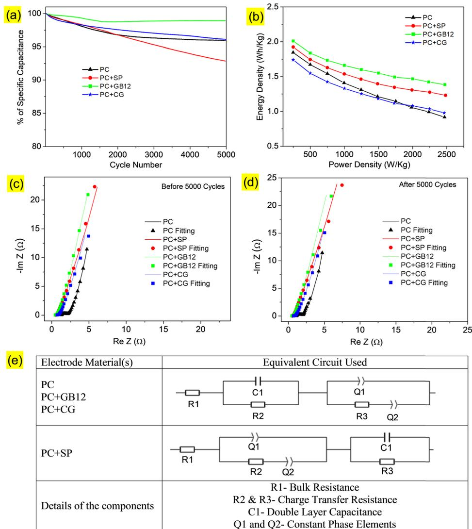
Fig. 6 Cycling stability of the supercapacitors, without conductive carbon (PC), Super P C65, GB12, and commercial graphene (CG) at a current density of  $10 \text{ A g}^{-1}$  (a); Ragone plot describing specific energy and power densities of supercapacitors (b); Nyquist plots of the supercapacitors before (c) and after 5000 cycles (d); and the equivalent circuit used to fit the impedance data (e).
