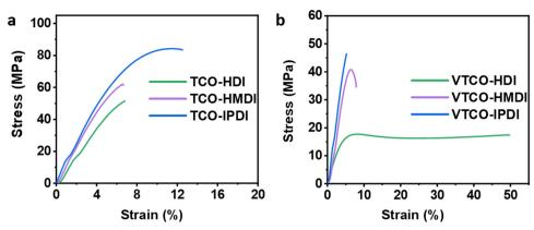
Fig. 6 Representative stress-strain curves of (a) TCO-NCO and (b) VTCO-NCO.
