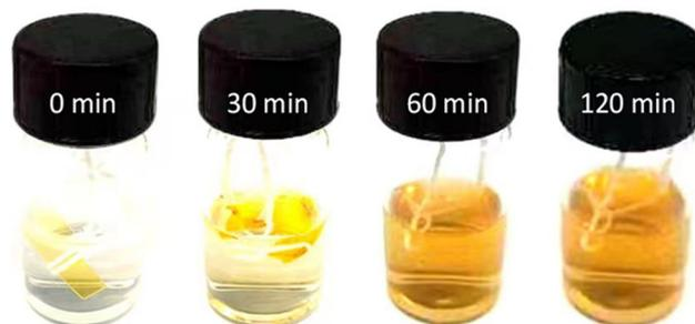
Fig. 9 Degradation process of VTCO-IPDI at different times in a 1 M HCl H<sub>2</sub>O/HFP (1/9, v/v) solution.
