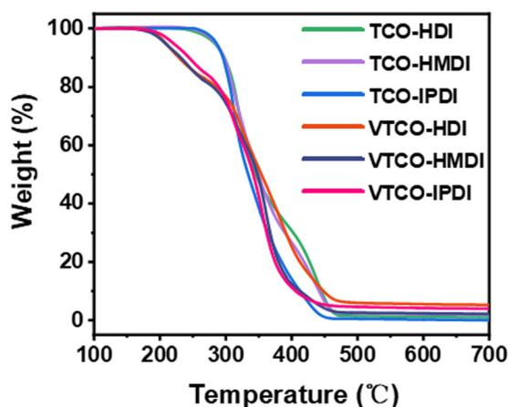
Fig. 4 TGA curves of TCO-NCO and VTCO-NCO.
