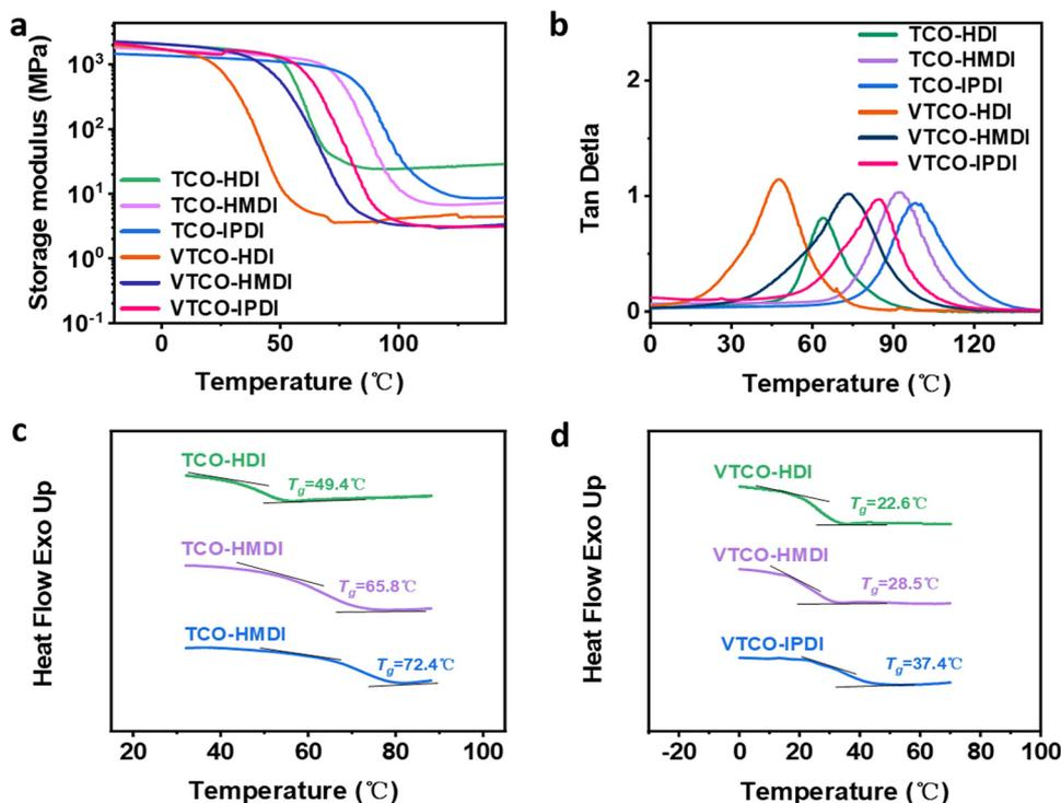
Fig. 3 (a) Storage modulus and (b) tan  $\delta$  as a function of temperature for TCO-NCO and VTCO-NCO by DMA. (c) DSC curve of TCO-NCO. (d) DSC curve of VTCO-NCO.
