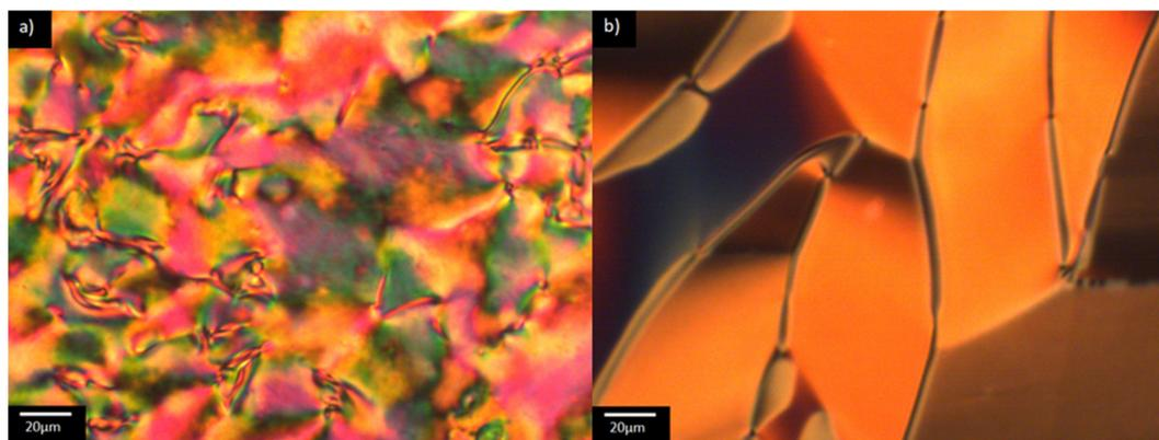
**Fig. 9** Polarised optical microscope textures observed for **O6**: (a) highly birefringent texture of the  $N_F$  phase viewed between untreated glass slides at 125 °C; (b) banded texture of the  $N_F$  phase in a cell treated for planar alignment at 125 °C.
