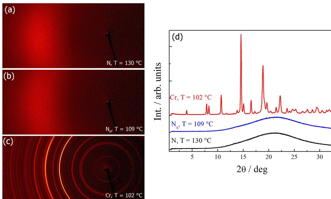
Fig. 7 X-ray diffraction patterns of compound **S1** in the (a) N phase; (b)  $N_x$  phase and (c) crystalline solid phase. (d) Intensity profiles of the X-ray patterns of the N phase (black line),  $N_x$  phase (blue line) and crystalline solid phase (red line).
