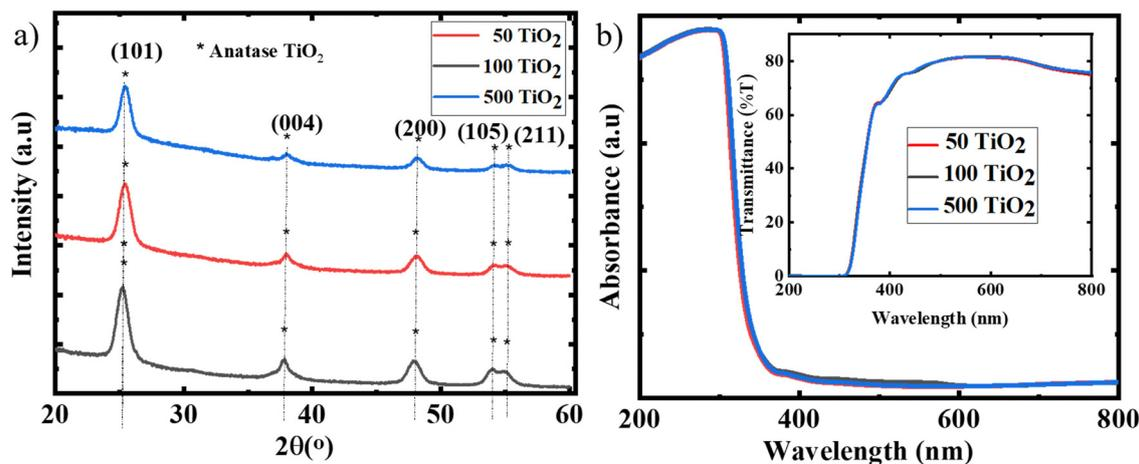
Fig. 2 (a) XRD spectra and (b) absorption spectra with transmission spectra of 50 TiO<sub>2</sub>, 100 TiO<sub>2</sub> and 500 TiO<sub>2</sub> as the inset image.
