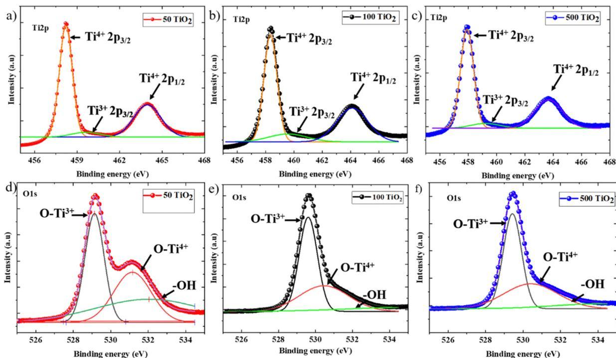
Fig. 6 (a)–(c) Ti2p XPS spectra and (d)–(f) O1s XPS spectra of 50 TiO<sub>2</sub>, 100 TiO<sub>2</sub> and 500 TiO<sub>2</sub>.
