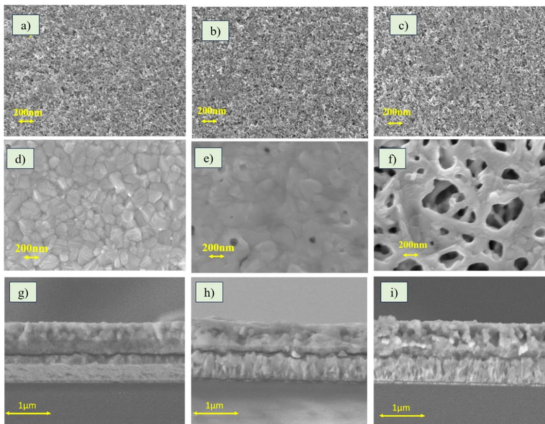
Fig. 3 FE-SEM surface morphology images of (a) 50 TiO<sub>2</sub>, (b) 100 TiO<sub>2</sub>, (c) 500 TiO<sub>2</sub>, (d) MaPbI<sub>3</sub> film on 50 TiO<sub>2</sub>, (e) MaPbI<sub>3</sub> film on 100 TiO<sub>2</sub> and (f) MaPbI<sub>3</sub> film on 500 TiO<sub>2</sub>, and cross section image of MaPbI<sub>3</sub> film on (g) 50 TiO<sub>2</sub>, (h) 100 TiO<sub>2</sub> and (i) 500 TiO<sub>2</sub>.
