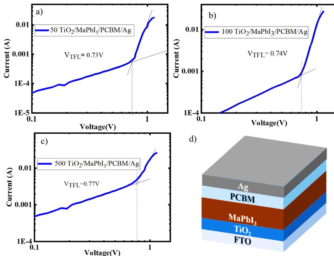
Fig. 4 Trap density and electron mobility calculations from IV spectra using the SCLC method for MaPbI<sub>3</sub> deposited on (a) 50 TiO<sub>2</sub>, (b) 100 TiO<sub>2</sub> and (c) 500. (d) Schematic diagram of the electron only device with device architecture TiO<sub>2</sub>/MaPbI<sub>3</sub>/PCBM/C.
