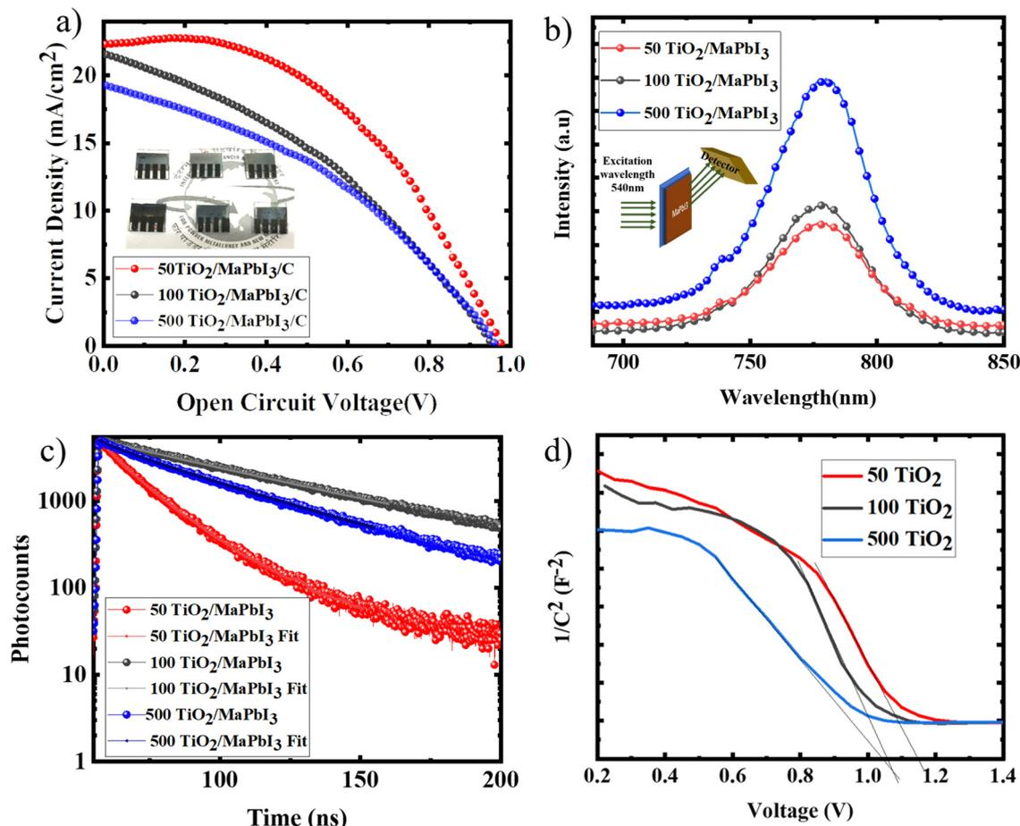
Fig. 7 (a) IV characteristics of CPSCs with 50 TiO<sub>2</sub>, 100 TiO<sub>2</sub> and 500 sintered TiO<sub>2</sub> as the ETL; (b) PL spectra and (c) TRPL spectra of MaPbI<sub>3</sub> films deposited on 50 TiO<sub>2</sub>, 100 TiO<sub>2</sub> and 500 sintered TiO<sub>2</sub>. (d) Mott-Schottky analysis at 1 kHz for the TiO<sub>2</sub>/MaPbI<sub>3</sub> carbon heterojunction solar cell.
