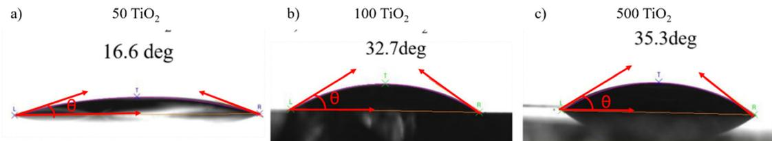
Fig. 5 Contact angle measurements of (a) 50 TiO<sub>2</sub>, (b) 100 TiO<sub>2</sub>, and (c) 500 TiO<sub>2</sub>.
