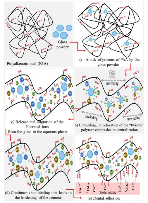
Fig. 3 Different mechanisms for the formation of glass ionomer cement.
