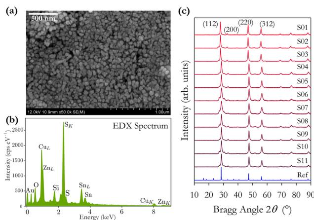
**Fig. 1** (a) SEM image of sample S01 at 50k magnification. Average particle size is  $51 \pm 9$  nm. The domain size inferred from XRD data is  $41.7 \pm 1.9$  nm. (b) EDX spectrum of sample S01 indicating a Cu-poor, Zn-rich composition. (c) X-ray diffraction spectra for as-synthesised nanocrystal samples S01–S11. For comparison, the reference plot for kesterite Cu<sub>2</sub>ZnSnS<sub>4</sub> (PDF 00-026-0575) is also shown.
