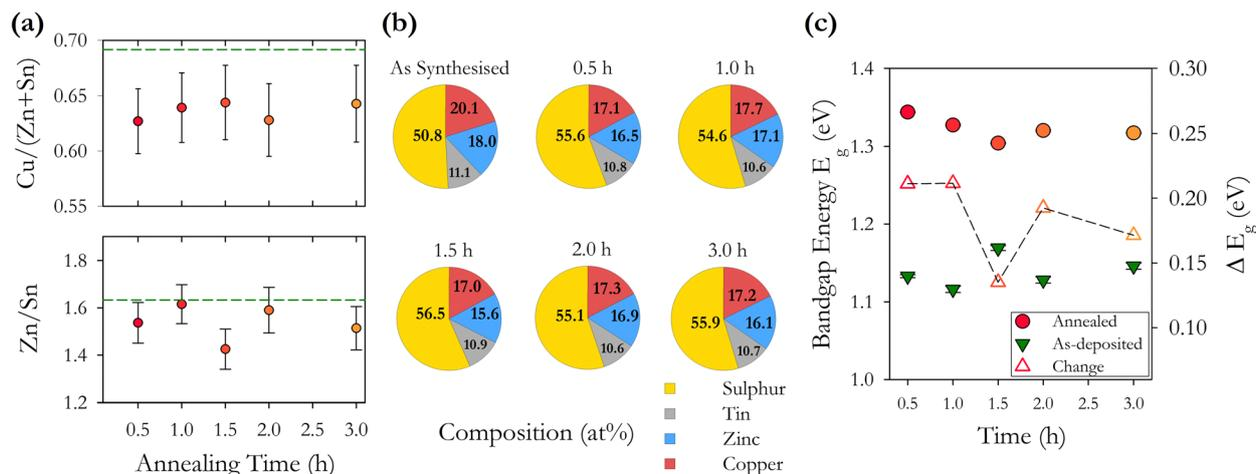
**Fig. 9** (a) Cation ratios Cu/(Zn + Sn) and Zn/Sn as a function of annealing time at 500 °C. The horizontal line shows the as-synthesised CZTS particles. (b) Normalised composition of as-synthesised CZTS particles and CZTS films annealed at 500 °C for varying times. (c) Variation in energy band gap  $E_g$  for as-deposited films and annealed films as a function of annealing time at 500 °C. The change in  $E_g$  with annealing is shown as an open triangle  $\Delta$ , the dashed line is a guide.
