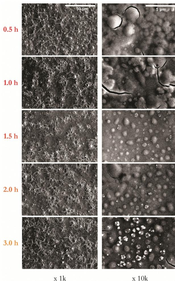
Fig. 8 Series of representative SEM images as a function of annealing at 500 °C with time from 0.5–3.0 hours shown at magnifications of 1k and 10k.
