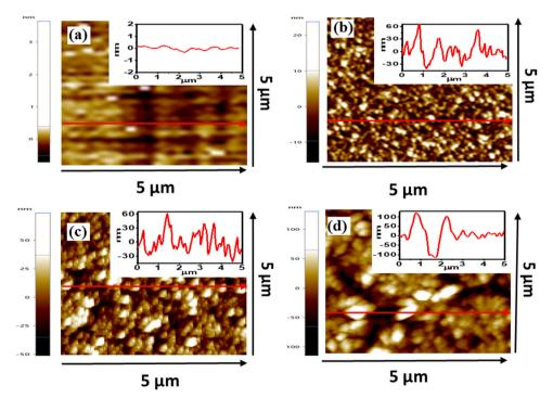
Fig. 2 Atomic force microscopy (AFM) images of (a) silicon, (b) ZnO nano-flowers, (c) ZnO nanoneedles, and (d) ZnO nanofibers. Inset shows the height profile of respective line drawn in an image
