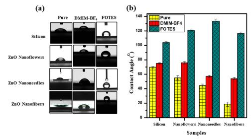
Fig. 3 (a) The optical images of a 5 µL water droplet standing on different samples with various surface morphologies. (b) Variation of the contact angle on silicon and all other nanostructured surfaces with different types of coatings. DMIM-BF4 is an imidazolium based ionic liquid and FOTES is a low energy hydrophobic material. The results of a flat silicon surface are compared with those of the surfaces covered with different nanostructures formed by ZnO
