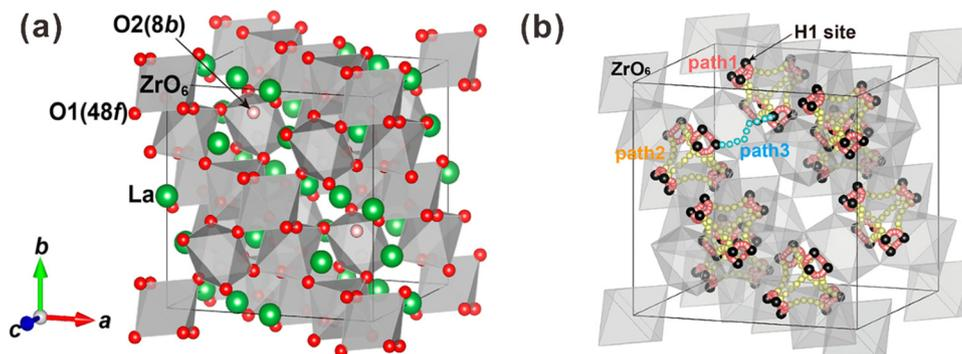
Fig. 6 (a) Pyrochlore crystal structure of  $\text{La}_2\text{Zr}_2\text{O}_7$ , where the green and red balls are La and O ions, and the grey octahedrons are  $\text{ZrO}_6$  units. (b) Conduction route of protons in  $\text{La}_2\text{Zr}_2\text{O}_7$ . Reprinted with permission,<sup>90</sup> Copyright [2015] American Chemical Society.
