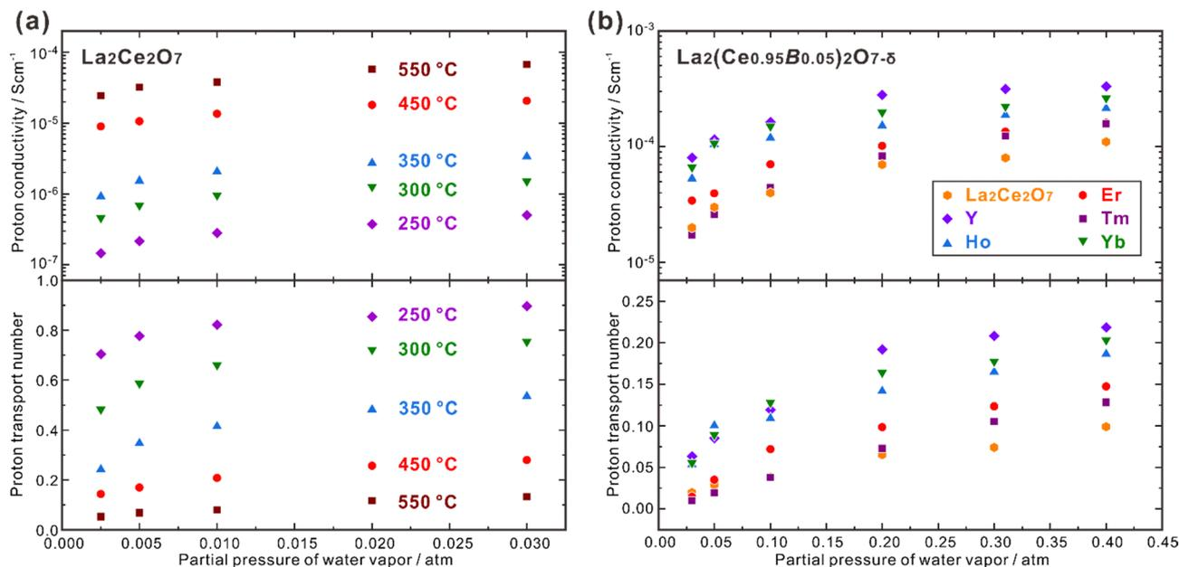
Fig. 4 Proton conductivity and proton transport number of (a)  $\text{La}_2\text{Ce}_2\text{O}_7$  in wet air,<sup>76</sup> and (b)  $\text{La}_2(\text{Ce}_{0.95}\text{B}_{0.05})_2\text{O}_{7-\delta}$  ( $\text{B} = \text{Y}, \text{Ho}, \text{Er}, \text{Tm}$  and  $\text{Yb}$ ) at 600 °C in wet oxygen plotted against  $p_{\text{H}_2\text{O}}$ .<sup>75</sup>
