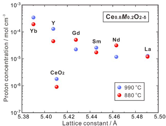
Fig. 3 Proton concentration in undoped CeO<sub>2</sub> and Ce<sub>0.8</sub>M<sub>0.2</sub>O<sub>2-δ</sub> (M = Y, La, Nd, Sm, Gd, Yb) after annealing at 880 and 990 °C in a wet atmosphere ( $p_{\text{H}_2\text{O}} = 0.03$  atm).<sup>62</sup>
