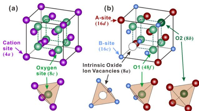
Fig. 1 (a) Fluorite and (b) pyrochlore crystal structures.
