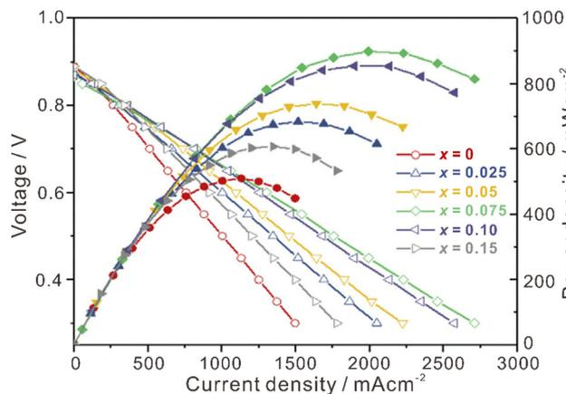
Fig. 10 Performance of fuel cells at 700 °C using  $(\text{La}_{1-x}\text{Mg}_x)_2\text{Ce}_2\text{O}_{7-\delta}$  as the electrolyte. Reprinted with permission,<sup>110</sup> Copyright [2019] Elsevier.
