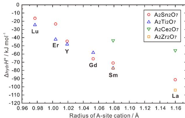
Fig. 8 Calculated hydration enthalpies for pyrochlore structured  $\text{A}_2\text{B}_2\text{O}_7$  (B = Ti, Sn, Zr, Ce).<sup>108</sup>
