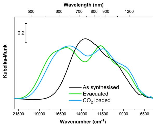
Fig. 9 Diffuse reflectance optical spectra of Cu-EtP collected on the as synthesised material, upon evacuation at 393 K and after contacting the evacuated material with CO<sub>2</sub> (ca. 0.5 bar).
