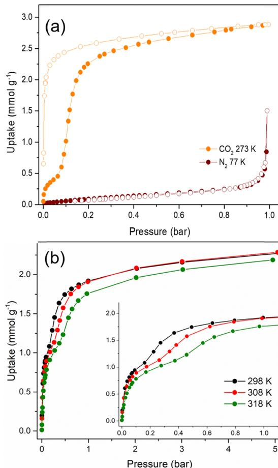
**Fig. 2** Low pressure N<sub>2</sub> (77 K, wine) and CO<sub>2</sub> (273 K, orange) adsorption/desorption isotherms (a) and high pressure CO<sub>2</sub> adsorption isotherms collected at 298 K (black), 308 K (red) and 318 K (green) (b). The isotherms were collected using 60 s of equilibration time.
