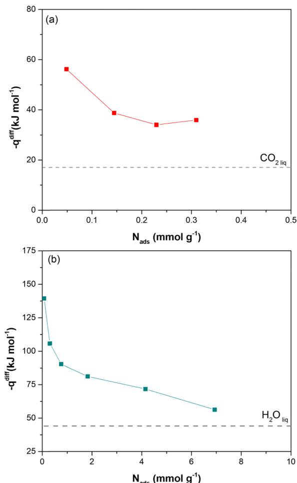
Fig. 3 Differential molar adsorption heat curves related to the adsorption of CO<sub>2</sub> at 308 K (a) and H<sub>2</sub>O at 303 K (b). The dotted horizontal line represents the standard molar heat of liquefaction of CO<sub>2</sub> and H<sub>2</sub>O (17 kJ mol<sup>-1</sup> and 44 kJ mol<sup>-1</sup>, respectively).
