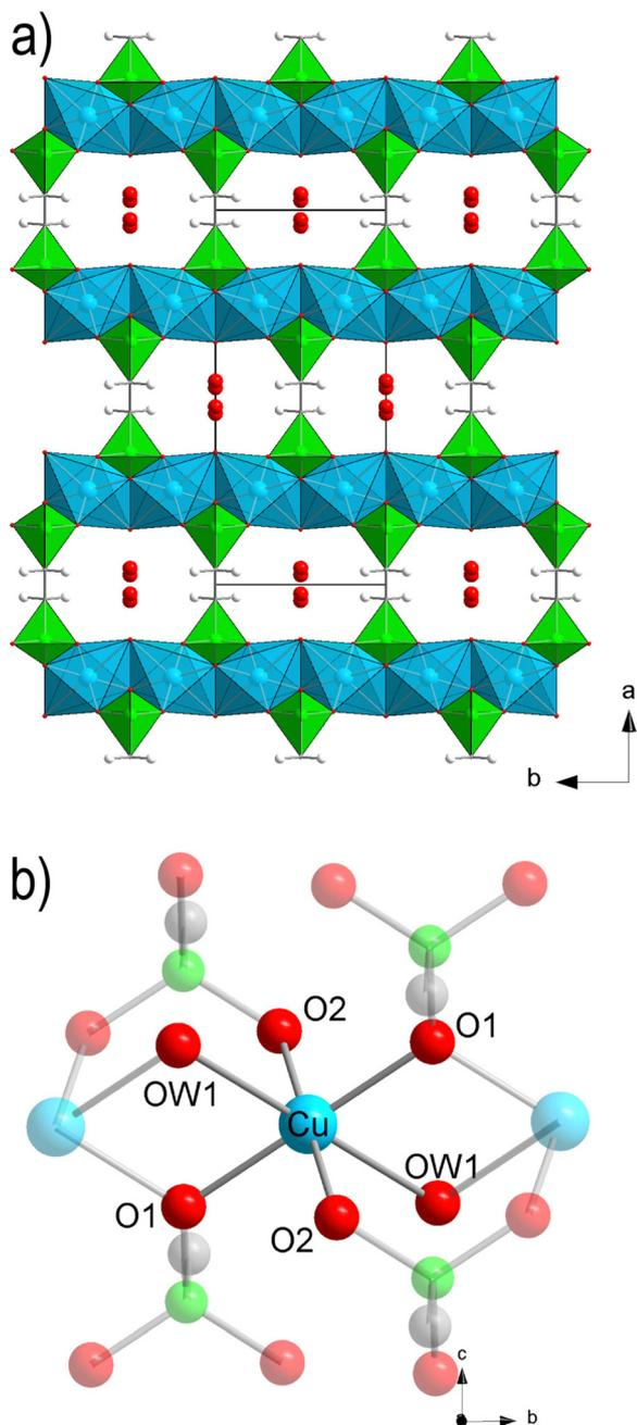
**Fig. 1** Polyhedral representation of the crystal structure of as synthesised Cu-EtP, viewed along the *c* axis (a) and detail of the local connectivity around the Cu<sup>II</sup> atoms (b, atoms not directly connected to the central Cu are shaded to highlight the coordination sphere of the central atom). Colour code: Cu, cyan; P, green; C, grey; O, red; H, white.
