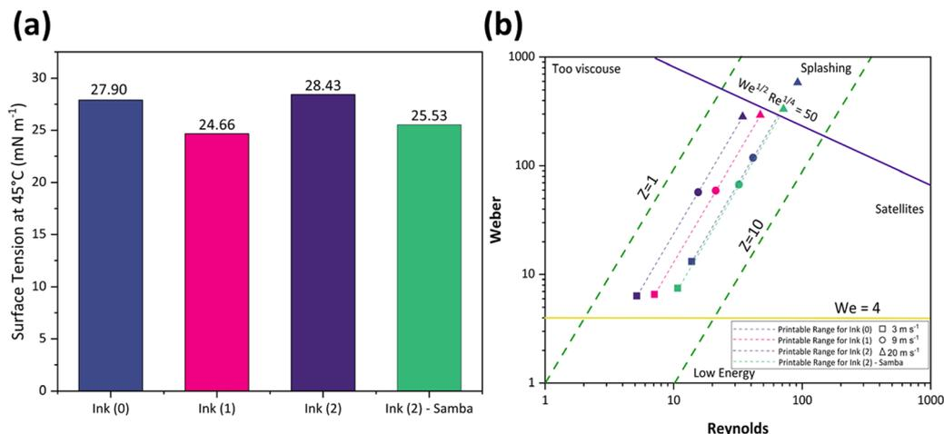
Fig. 3 Ink characterization plots. (a) Surface tension measurement of Ink (0), Ink (1), Ink (2), and Ink (2) – Samba at the printing temperature (45 °C). (b) Derby diagram for Ink (0), Ink (1), Ink (2), and Ink (2) – Samba at the printing temperature (45 °C).
