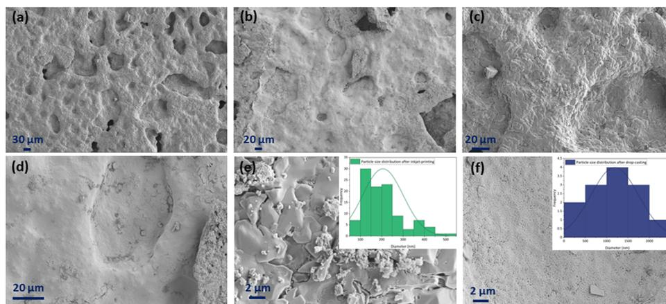
**Fig. 10** Surface SEM images of (a), (c) and (e) 100-layer and (b), (d) and (f) drop-cast porous NLK–GDC symmetric cells in 185× (a and b), 687× (c and d), and 4.15k× (e and f) magnifications. The insets of (e) and (f) figures are the particle size distributions of CuFe<sub>2</sub>O<sub>4</sub> particles on the surface of the inkjet-printed and drop-cast samples, respectively, analyzed using ImageJ software.
