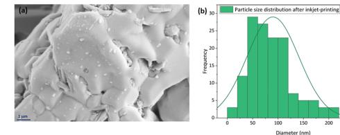
Fig. 11 (a) Surface SEM image with a high magnification of 8.66k× from the 100-layer inkjet-printed sample and (b) CuFe<sub>2</sub>O<sub>4</sub> nanoparticle size distribution on its surface, analyzed using ImageJ software.
