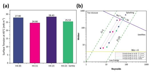
Fig. 3 Ink characterization plots. (a) Surface tension measurement of Ink (0), Ink (1), Ink (2), and Ink (2) – Samba at the printing temperature (45 °C). (b) Derby diagram for Ink (0), Ink (1), Ink (2), and Ink (2) - Samba at the printing temperature (45 °C).
