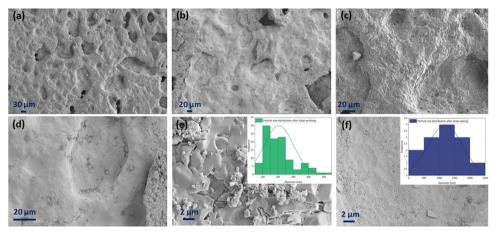
Fig. 10 Surface SEM images of (a), (c) and (e) 100-layer and (b), (d) and (f) drop-cast porous NLK-GDC symmetric cells in 185× (a and b), 687× (c and d), and 4.15kx (e and f) magnifications. The insets of (e) and (f) figures are the particle size distributions of CuFe<sub>2</sub>O<sub>4</sub> particles on the surface of the inkjetprinted and drop-cast samples, respectively, analyzed using ImgaeJ software.
