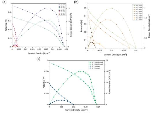
Fig. 9 IV and IP curves of (a) 100-layer inkjet-printed and (b) drop-cast full fuel cells with Ink (2) – Samba at 500-650 °C (H<sub>2</sub> with 5 L min<sup>-1</sup> and air with 12.5 L min<sup>-1</sup> were supplied on the anode and cathode sides, respectively), and (c) comparison of inkjet-printed and drop-cast full fuel cells with Ink (2) – Samba at 650 °C.
