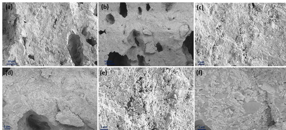
Fig. 12 Cross-sectional SEM images of (a), (c) and (e) 100-layers and (b), (d) and (f) drop-cast porous NLK–GDC symmetric cells in 1.23k $\times$  (a and b), 3.71k $\times$  (c and d), and 9.77k $\times$  (e and f) magnifications.
