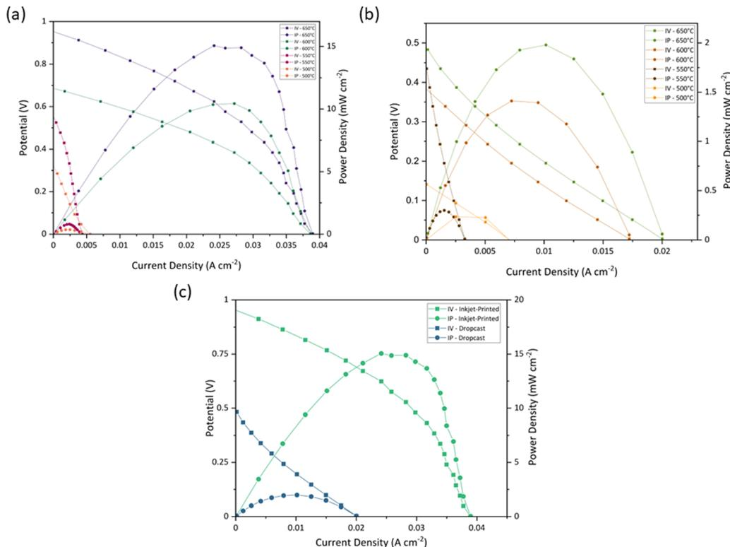
**Fig. 9** IV and IP curves of (a) 100-layer inkjet-printed and (b) drop-cast full fuel cells with Ink (2) – Samba at 500–650 °C ( $\text{H}_2$  with 5 L  $\text{min}^{-1}$  and air with 12.5 L  $\text{min}^{-1}$  were supplied on the anode and cathode sides, respectively), and (c) comparison of inkjet-printed and drop-cast full fuel cells with Ink (2) – Samba at 650 °C.
