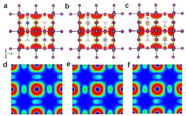
Fig. 5 Sum of the electron density of the degenerated CBMs of the proposed 3D perovskites with complex ions. Isosurface plot of the 3D CBM electron density (isovalue =  $0.0008 \text{ e Bohr}^{-3}$ ) of  $\text{Cu}(\text{NH}_3)_2\text{Pbl}_3$  (a),  $\text{Ag}(\text{NH}_3)_2\text{Pbl}_3$  (b), and  $\text{Au}(\text{NH}_3)_2\text{Pbl}_3$  (c). 2D CBM charge density maps on the (101) plane of  $Cu(NH_3)_2PbI_3$  (d),  $Ag(NH_3)_2PbI_3$  (e) and  $Au(NH_3)_2PbI_3$  (f).
