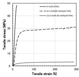
Fig. 7 Typical tensile stress-strain curves for polyamide 4 and Nmethylol polyamide 4 (degree of methylolation 4.5 mol%, 22.5 mol%)
