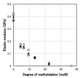
Fig. 9 Relationship between elastic modulus at hygroscopic equilibrium and degree of methylolation for N-methylol polyamide 4 (black filled circle: average of each lot, white open circle: average of each specimen for the same lot)
