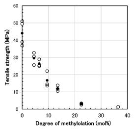
Fig. 8 Relationship between tensile strength and degree of methylolation for N-methylol polyamide 4 (black filled circle: average of each lot, white open circle: average of each specimen for the same lot).
