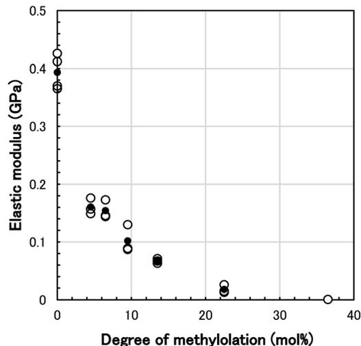
Fig. 9 Relationship between elastic modulus at hygroscopic equilibrium and degree of methylation for *N*-methylol polyamide 4 (black filled circle: average of each lot, white open circle: average of each specimen for the same lot).
