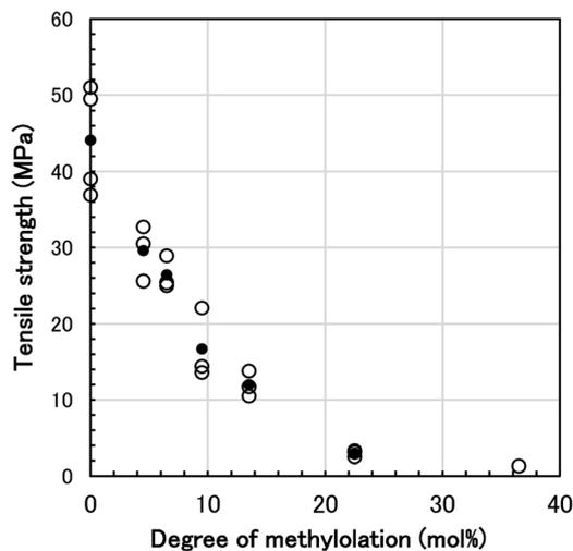
Fig. 8 Relationship between tensile strength and degree of methylation for *N*-methylol polyamide 4 (black filled circle: average of each lot, white open circle: average of each specimen for the same lot).
