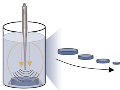
**Sonication labile PEG-based hydrogel system for biological component suspension and subsequent degradation**
