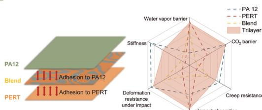
**A polyamide and polyethylene multilayer composite with enhanced barrier and mechanical properties at high temperature**
