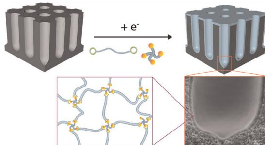
**Cathodic electrodeposition of polymer networks as ultrathin films on 3-D micro-architected electrodes**
