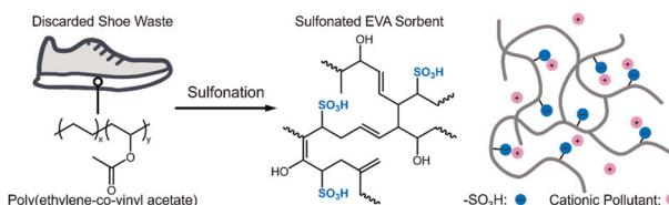
**Valorization of shoe sole waste into high-performance cationic dye sorbents via sulfonation**
