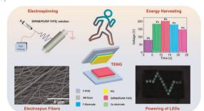
Triboelectric nanogenerator based on electrospun molecular ferroelectric composite nanofibers for energy harvesting
