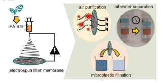
Bio-based electrospun polyamide membrane sustainable multipurpose filter membranes for microplastic filtration
